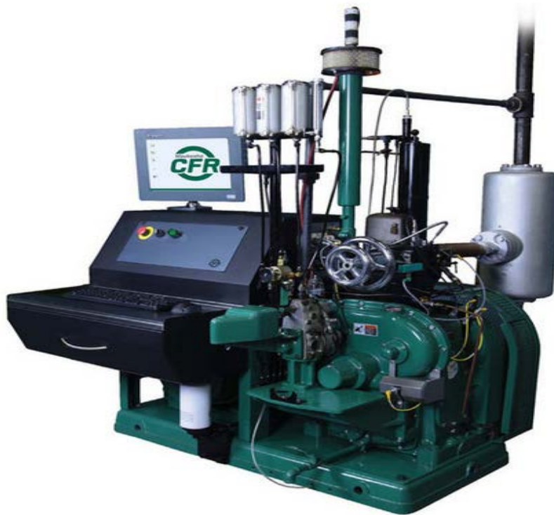
Figure 3-1: A Waukesha CFR F5 Diesel Test Engine
