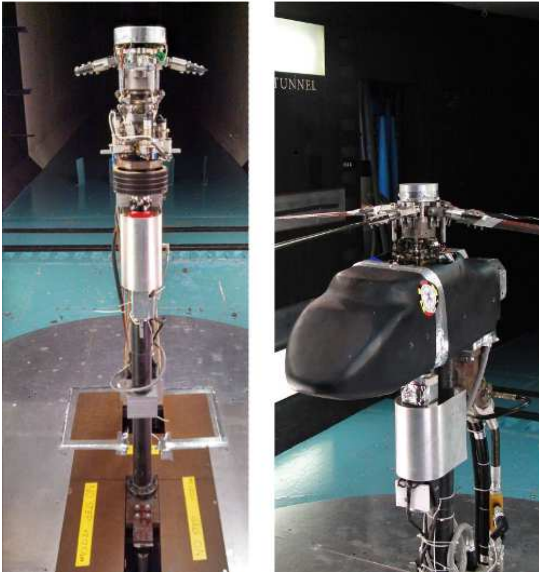
Figure 5.1: University of Maryland rotor in Glenn L. Martin wind tunnel.
