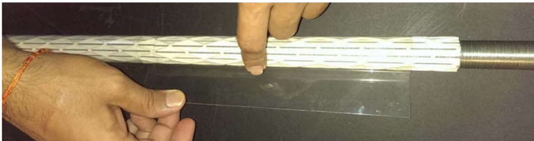
Figure 4-9: Transparent plastic sheet is wrapped around the manifold to stop the leakage
