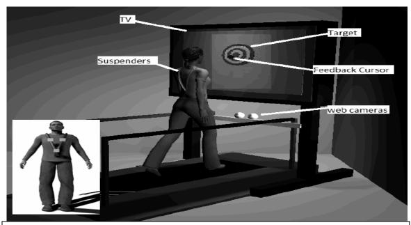
Figure 5-1. Illustration of the experimental set-up. Subjects walked on the treadmill in front of a wide screen TV. Center of mass displacement or trunk orientation was indicated by cursor motion over a bulls-eye target. Depicted is the feedback condition. The TV was turned off and covered with a cloth for the no-feedback condition.
