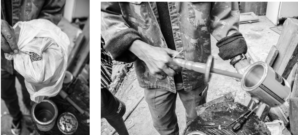
Figure 5 Making a maracá from tin can, ball bearings, and wooden handle.
