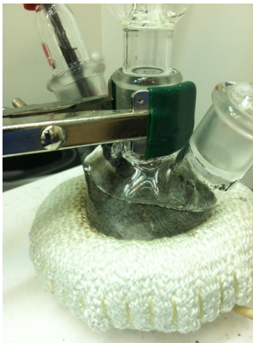
Figure 2.20) An image of the HNO 3 bath solution that hosts the acid reflux conducted to functionalize the surface of the carbon nanotubes.
