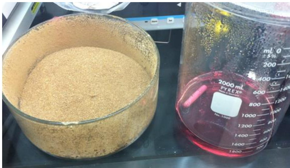
Figure 2.12) An image of the pink catalyst solution and the resulting brown powder catalyst after a combustion synthesis method.
