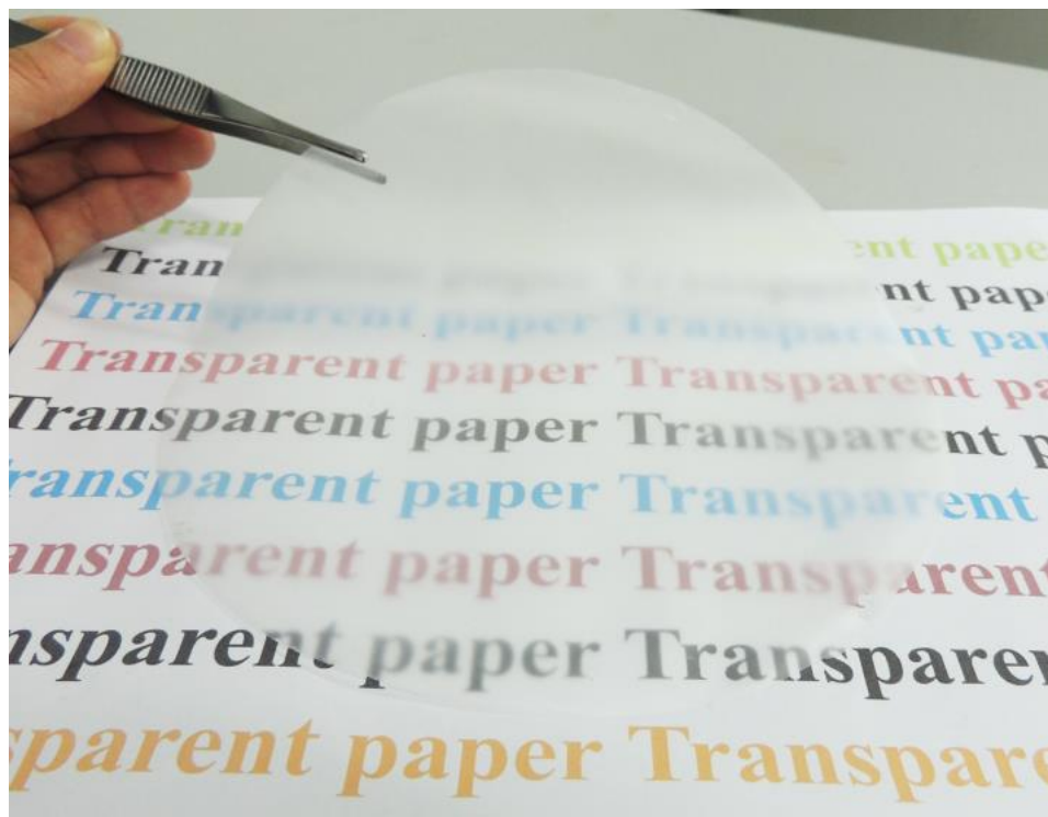
Figure 5.6) An image of transparent paper produced from TEMPO-oxidized wood fibers with a diameter of 20 cm. [152]
