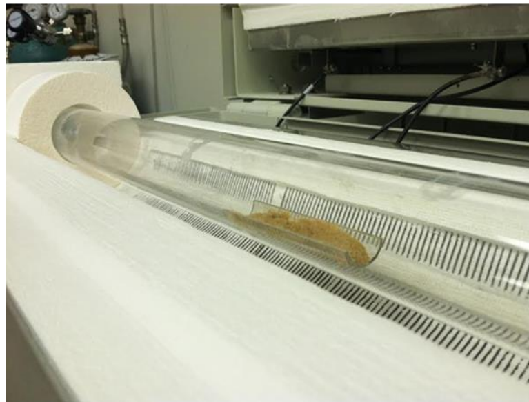
Figure 2.14) An image of the powder catalyst inserted into the quartz boat that is inserted into the tube furnace for the chemical vapor deposition growth of carbon nanotubes.
