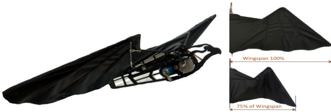
Figure 10: Active Wing Morphing Bio- inspired Research Platform a) Ornithopter Platform b) Extended Half Wingspan vs. Retracted Half Wingspan [39]
