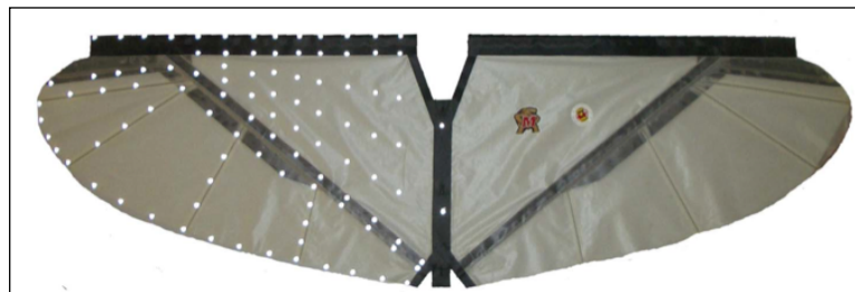
Figure 44: MSK004 wings with tracking markers [19]
