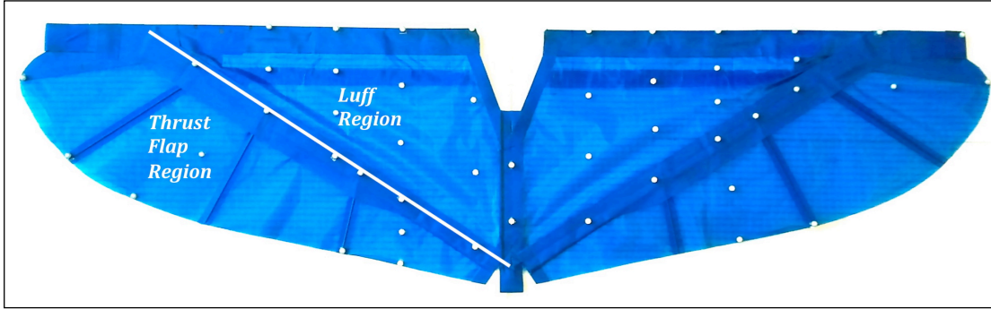
Figure 54: Asymmetric retro reflective markers on the wing (seen as white dots) and Wing tip Location (Marked in Red)
