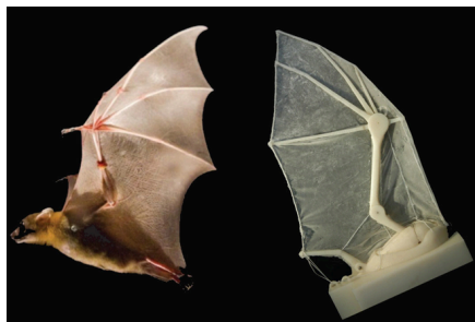
Figure 15: Brown University Robotic Bat Wing a) ABS 3 D Print b) Schematic [49]
