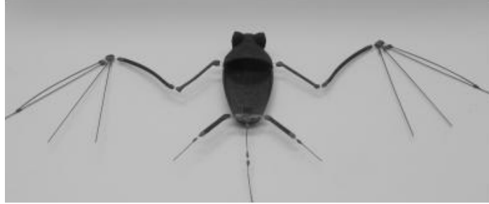
Figure 16: “Robo Bat”s the skeleton of the robotic bat uses shape-memory metal alloy that is superelastic for joints [50]
