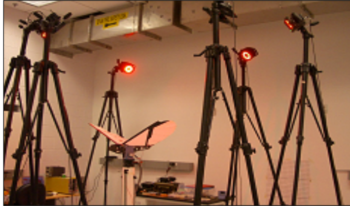
Figure 45: MSK004 and Vicon camera system for the measurement of ornithopter wing and configuration motions [19]
