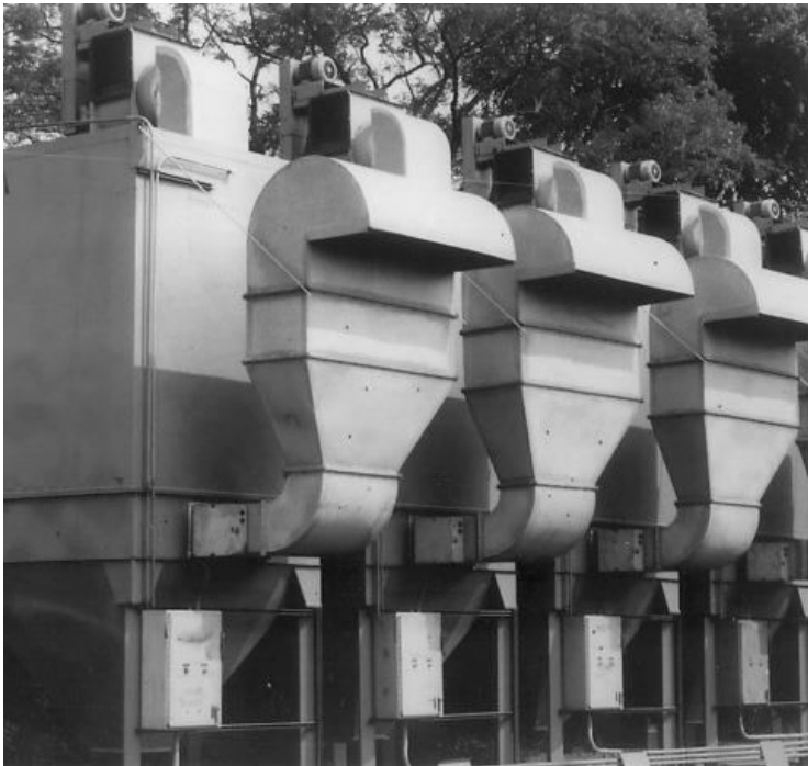
Figure 4.4 Baghouses used for SRM 1649b Urban Dust collection. Courtesy of Lane Sander.
