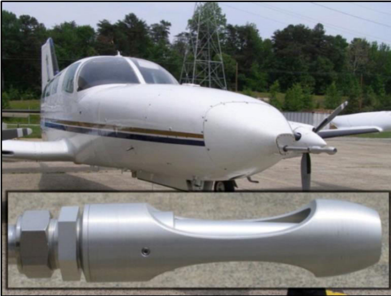
Figure 6.2 Shrouded inlet diffuser on Cessna 402. This inlet, purchased from Droplet Measurements, Boulder, CO, was mounted onto the Cessna 402 and used for RAMMPP data collection as of the Summer 2011 flying season.
