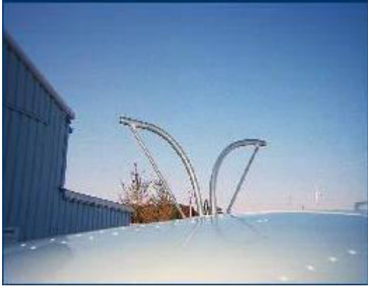
Figure 6.1 Piper Aztec roof mounted aerosol inlet. “Aztec Antlers” The aerosol inlet faces forward and the gas inlet faces aft. Aztec aerosol inlet was a 3 mm i.d. Swagelok Tube Fitting Connector attached to conductive tubing inserted into the forward facing (right side) antler shown above.
