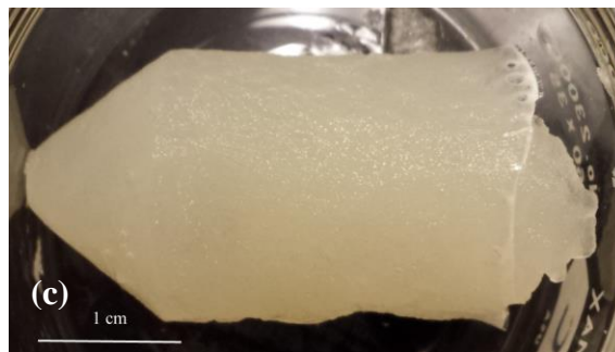
Figure 3.3. Visual observation after the fifth freeze-thaw cycle; WPI: XC of (5:0) (a), (5:0.25) (b), (5:0.5) (c)
