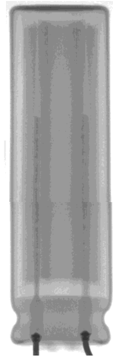
Figure 22: X-ray image of a good untested capacitor (C1)
