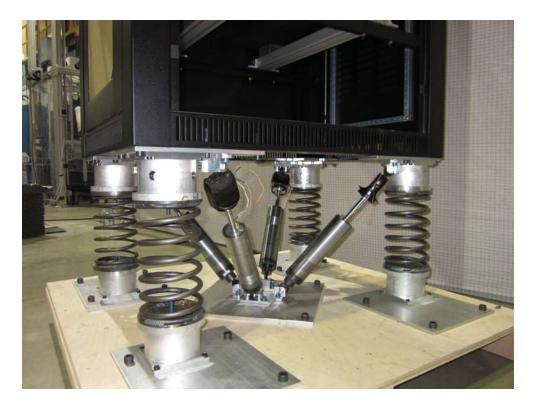
Figure 5.18: Pyramid configuration of suspension.
