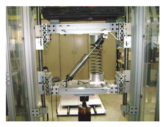
Figure 5.12: Vertical 1-DOF vibration test stand.
