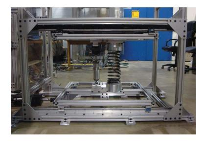
Figure 5.9: Lateral 1-DOF shake table test stand.
