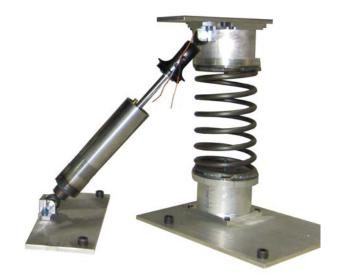
Figure 4.2: Single suspension leg.
