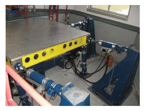
Figure 5.19: GW-NSF hydraulic shake table at George Washington University.
