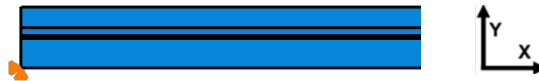
Figure 10. Pin displacement BC constraint along on the bottom left corner of the model
