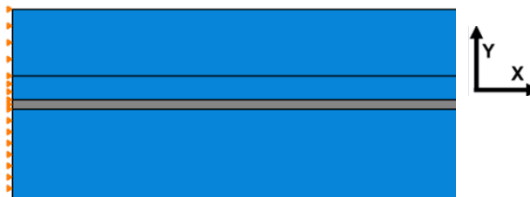
Figure 12. Displacement BC constraining the right end of the model in the horizontal x-axis
