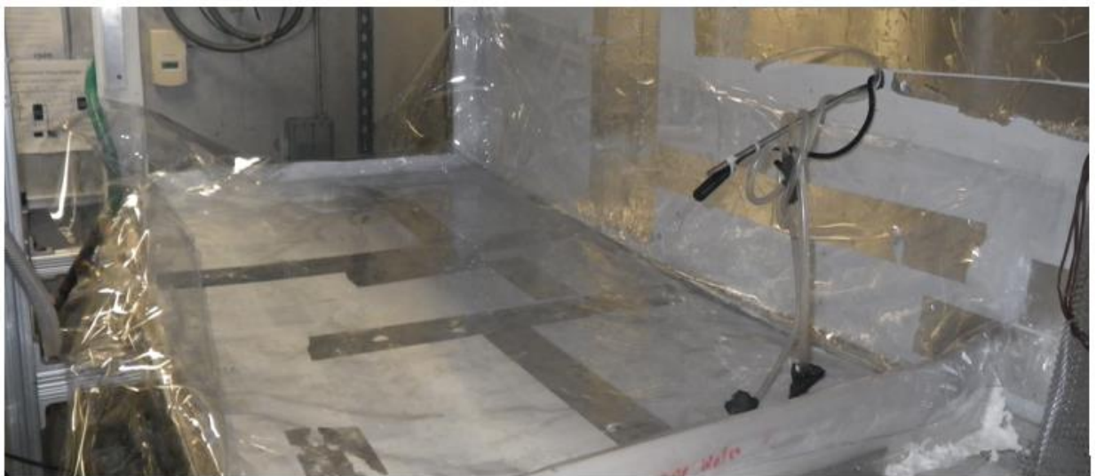
Figure 2.3: Plastic sheet is used to ensure collection of wetting water into the wetting water tank.
