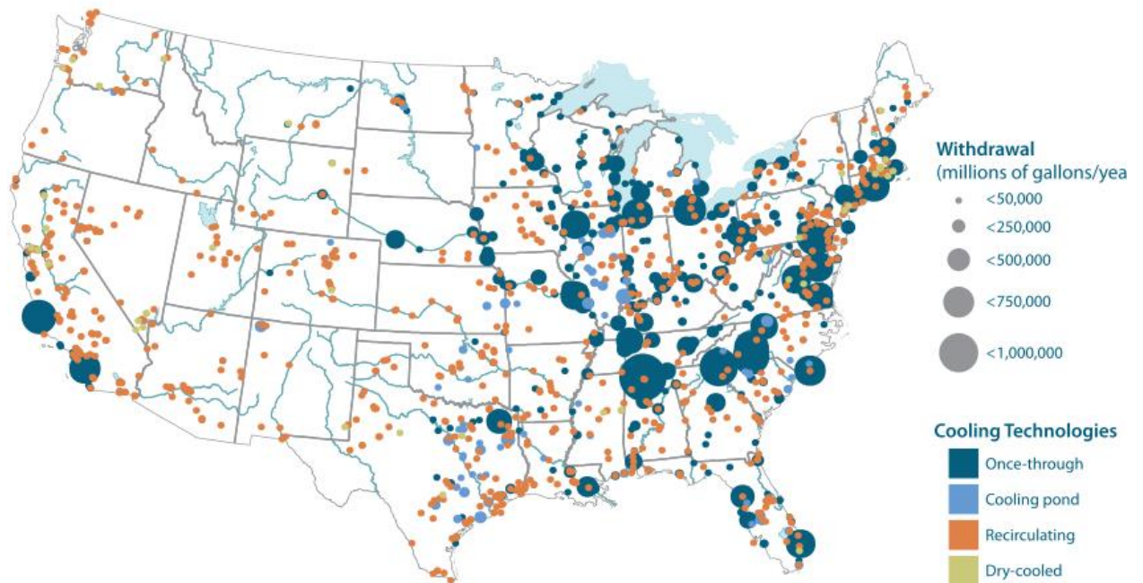
Figure 1.2: Condenser cooling technology and their water withdrawal rate within the power plant sector in US [Avery et al., 2011].
