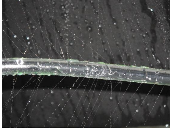
Figure 6.5: Uniform spray pattern obtained from plastic tube with holes in all directions.
