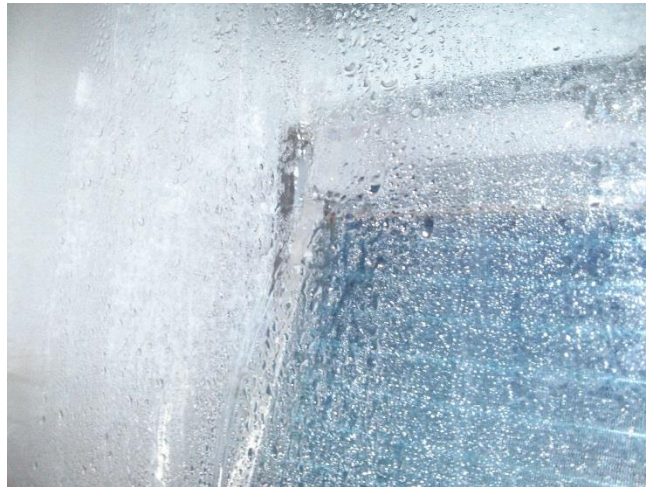
Figure 5.15: Unevaporated spray droplets deposited on visualization section plate at air outlet of experimental setup.
