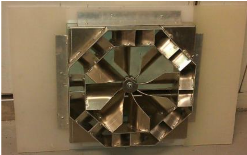
Figure 2.9: Air-mixer attached to polypropylene sheet, ready to be mounted in test section.
