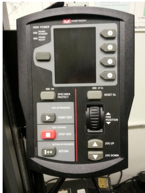
Figure 17.(a) Instron testing stand and (b) Instron control module
