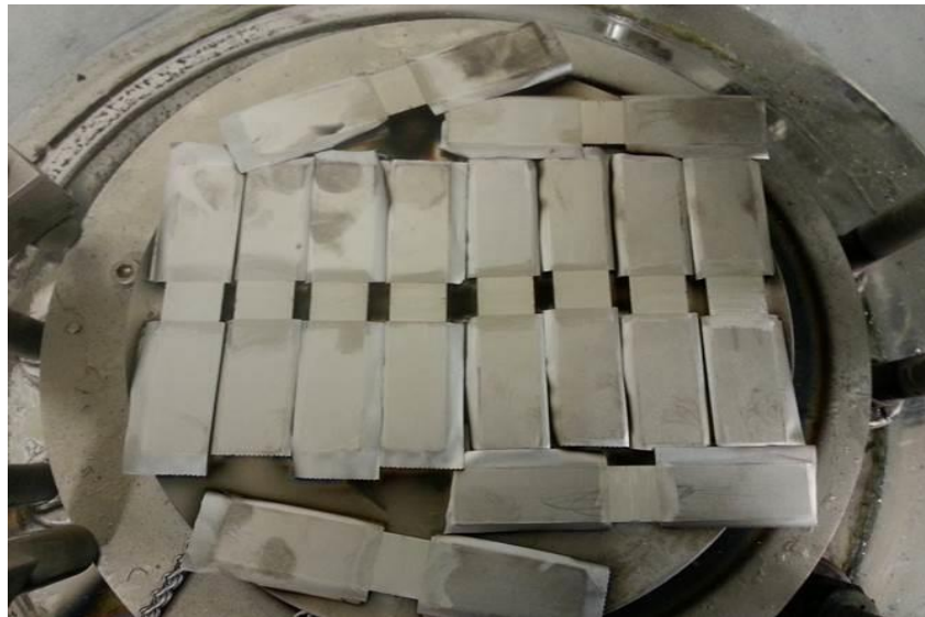
Figure 25. Aluminum deposition in vacuum chamber
