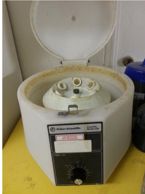
Figure 29. Centrifuge for mixing epoxy
