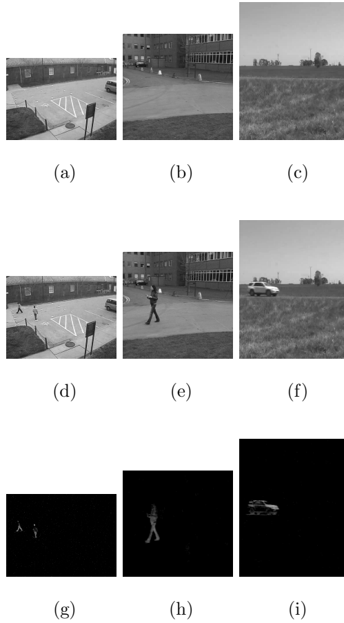
Figure 4.4: Example images from the marker_cam , PETS2009_S2L1 , and convoy2 (columns one, two, and three, respectively), video sequences. The first row contains the background images, the second row contains an image with both foreground and background components, and the third image contains the corresponding foreground component.
