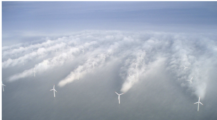
Figure 1.1: Photograph of the Horns Rev wind farm with visual illustration of aerodynamic interactions between turbines (notice the turbines amidst the condensation; photo courtesy Christian Steiness).
