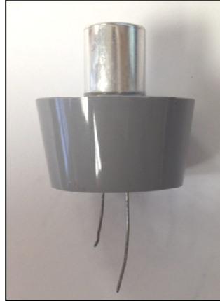
Figure 4: Encapsulated capacitor (potted capacitor)
