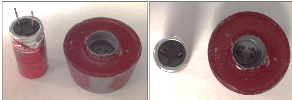
Figure 30: Dummy sample to observe dye penetration into the delaminations
