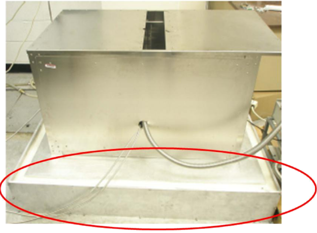
(b) Sand box and a granite sheet placed underneath the mu-metal (20 Hz cut-off)
