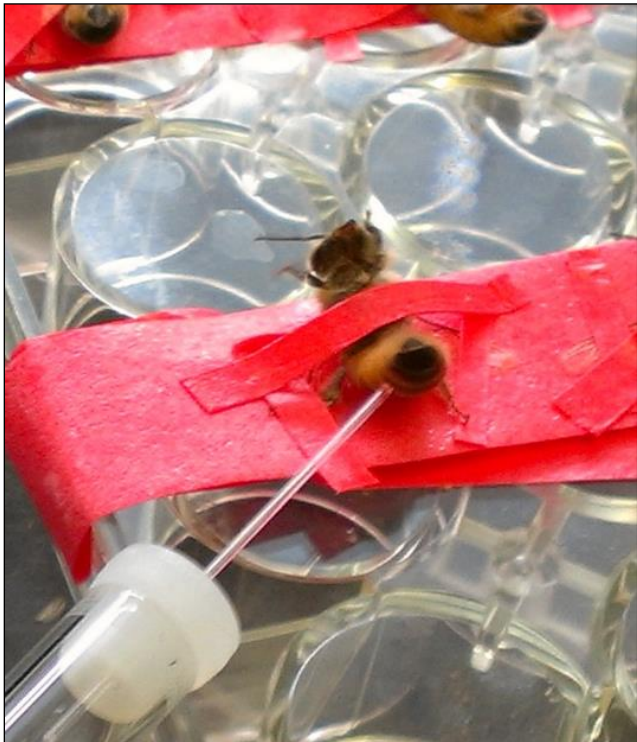
Figure 3: Removing hemolymph from the honey bees using a 1uL micro capillary tube.
