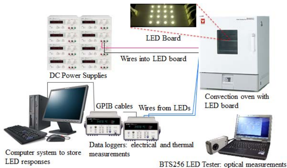
Figure 48 Overview of LED test setup.
