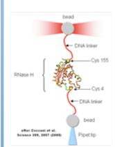
Figure 2. Optical tweezer set-up for protein folding experiments.
