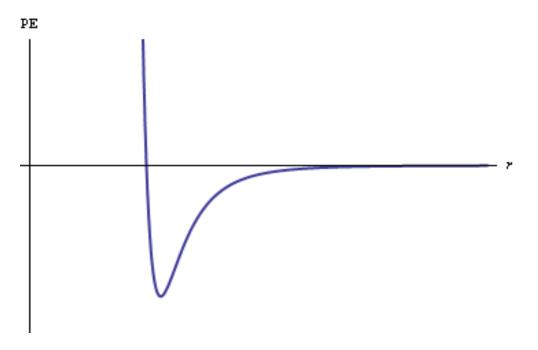
Figure 4.3a. The Lennard-Jones potential, approximating the potential energy associated with the interaction of two atoms, as a function of the distance (r) between the atoms.
