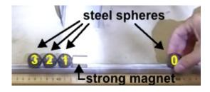
Figure 4.5. The Gauss gun.
