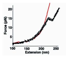
Figure 3. Data obtained when RNase H is explored via the optical tweezer set-up described above.
