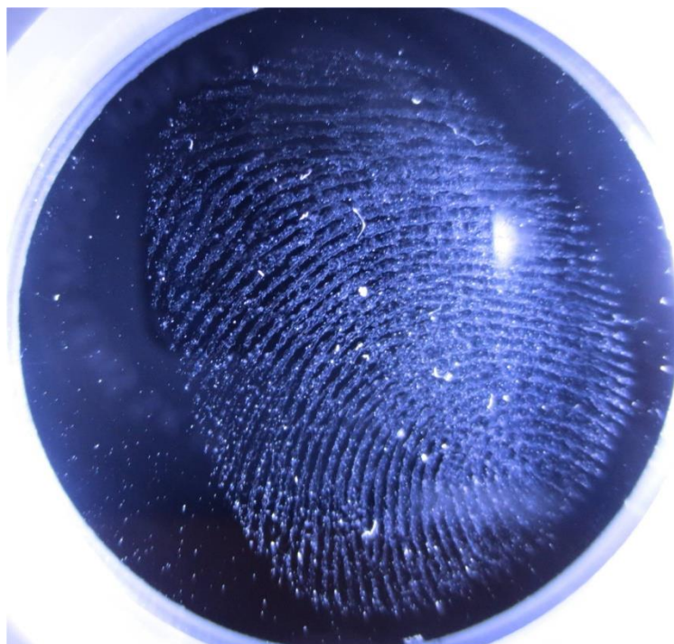
Figure 7.7 Optical image of a one year old fingerprint. Note that the ridges and valleys are still visibly distinguishable.
