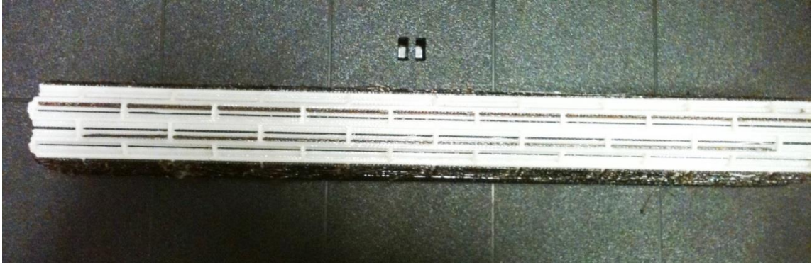
Figure 4-4: 3D printed manifold after printing is complete
