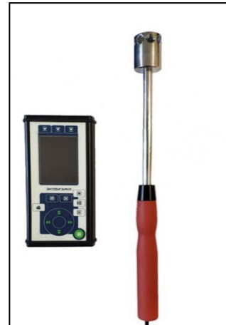
Fig. 3. Measuring device PZ-80 and the display unit Ecophysics-110A
