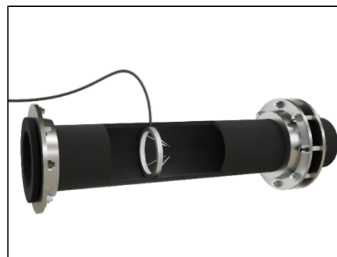
Fig. 1. 3-d model of the ionizer experimental setup
