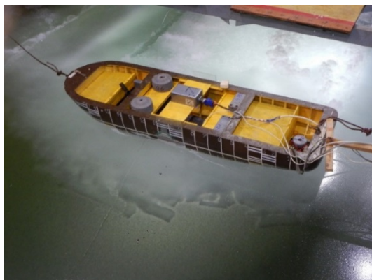
Fig. 6. Testing of the IRSPP model in the ice tank of the AARI during ice compression. (Photos by AARI)
