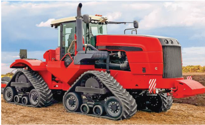
Fig. 2. Tractor with rubber metal crawler tracks.
