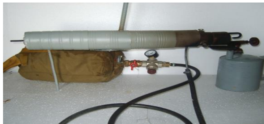
Fig. 4. Autonomous steam generator set, ready for operation (with protective cover and backpack).
