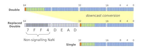
Figure 6.4: In-place downcast conversion and replacement
