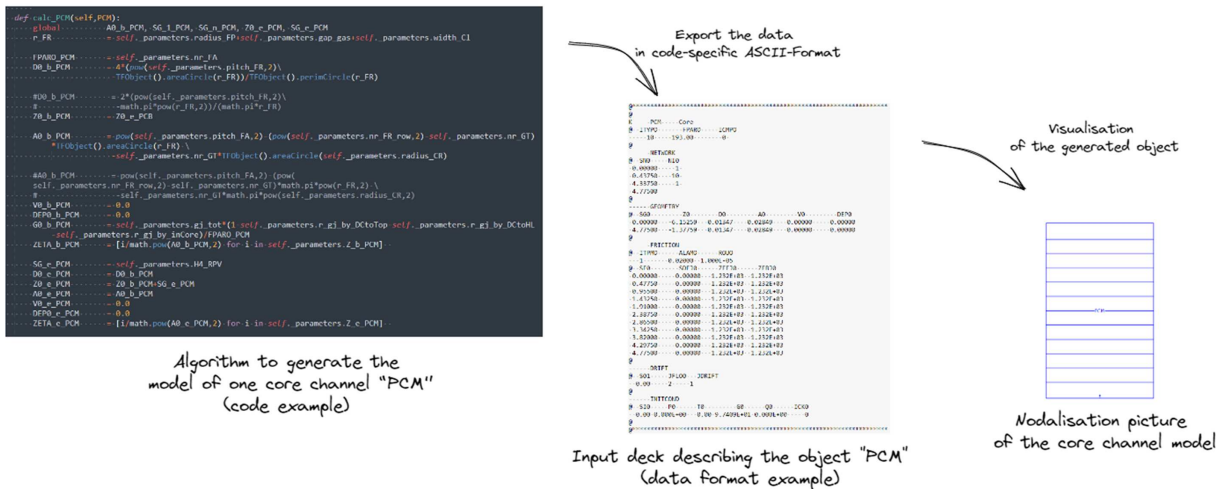
Fig. 8. Steps to generate one core channel model in ATHLET with the AMG tool.
