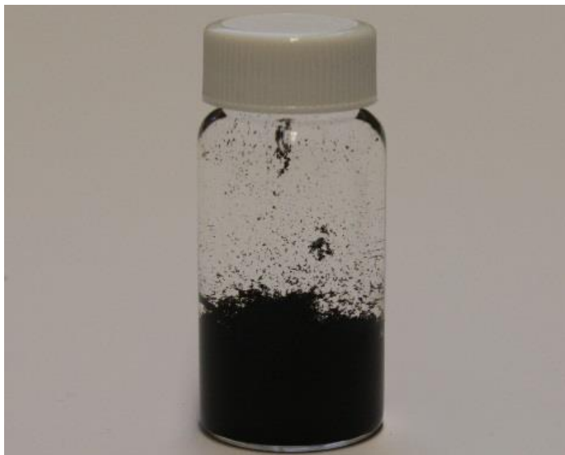
Figure 3.5. SWNT solution post-sonication. Without a surfactant, sucrose solution failed to disperse SWNTs during sonication.
