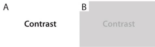
Figure 4.1. For printed text media, the contrast ratio tells the level of white to the level of black for the media and text respectively. The print in (A) has good contrast with black text on media. The off-white (light-gray) background and gray text give the print in (B) poor contrast.
