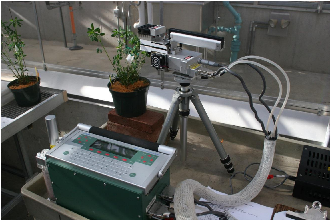
Figure 3.2: Licor 6400XT Photosynthesis meter clamped on an alfalfa, Medicago sativa , plant leaflet.
