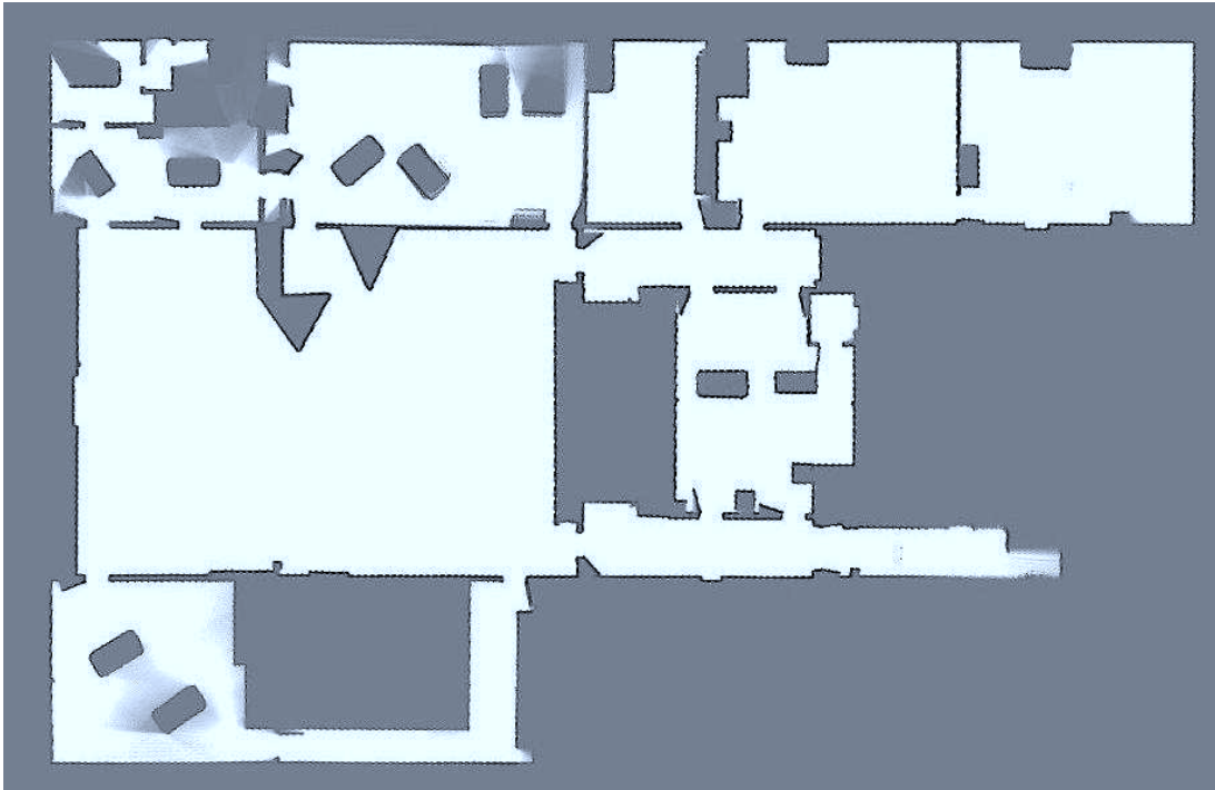
(a) Results by Andrew Howard et al. Occupancy grid color coded with grayscale for occupancy values between 0 and 1 (image copied from the online Radish dataset repository [85]).
