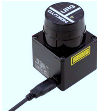
Figure 4.1: Hokuyo laser range scanner: URG 04LX-UG01.
