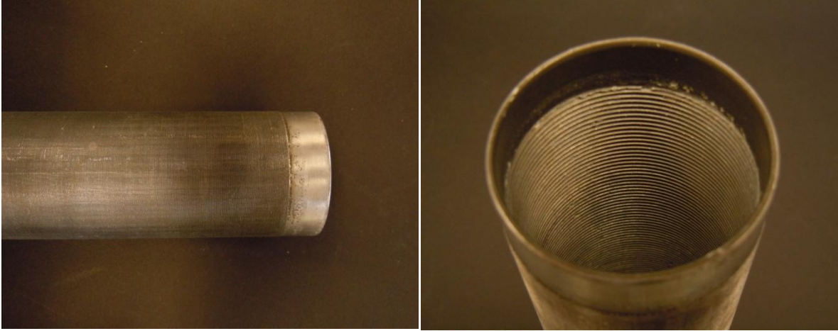
Figure 7 Refrigerant and Water Side Surfaces
