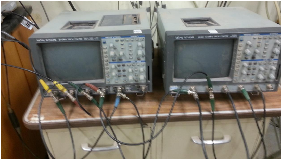
Figure 2.3: LeCroy oscilloscopes used for data acquisition
