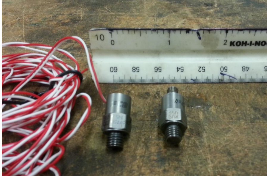
Figure 2.1: Accelerometers used for dynamic testing. Note the 50000g accelerometer (left) has the cable integrated into the system and the 5000g accelerometer (right) does not. The upper scale is in inches.
