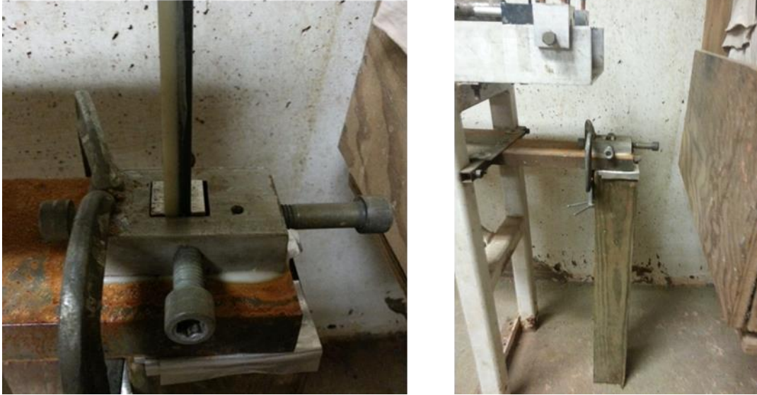
Figure 2.12: Cantilever support used for dynamic testing of polyurea coated beams
