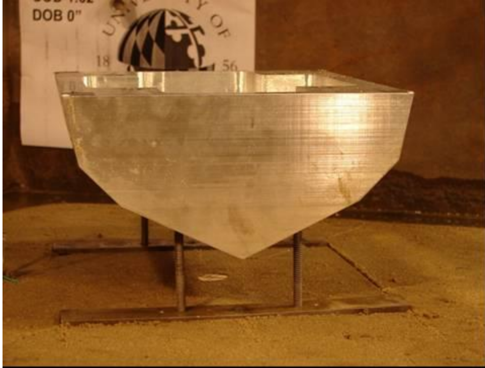
Figure 1.2: Example of a V-Shaped bottom as tested by the Dynamic Effects Lab [6]
