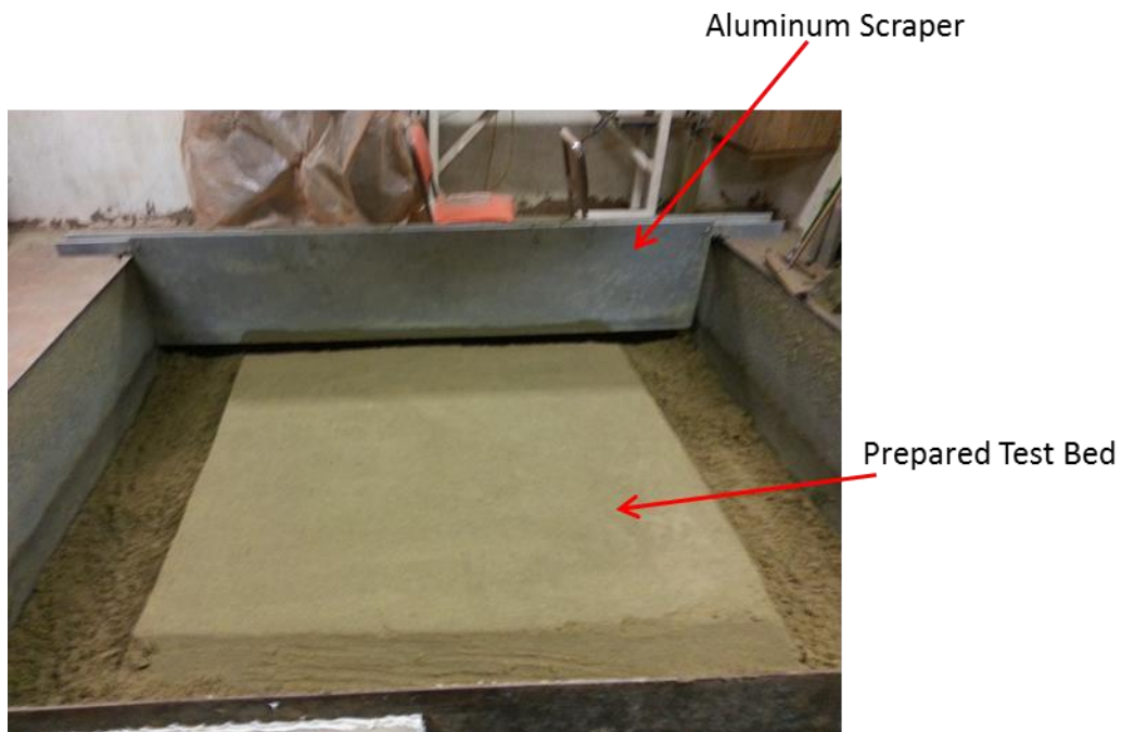
Figure 2.13: Prepared test bed with aluminum scraper resting along the backside
