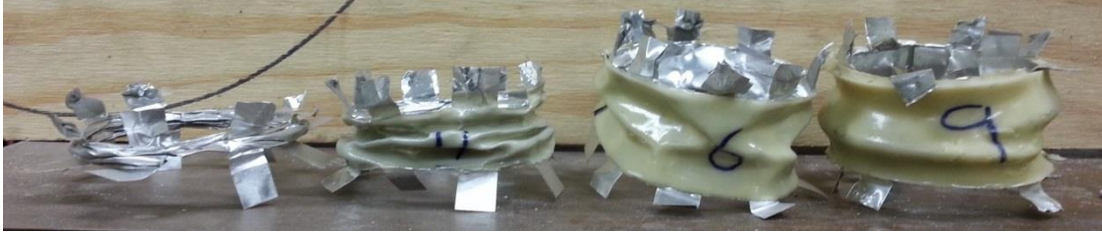
Figure 5.32: Front view of crushed cylinders increasing in polyurea mass from left to right
