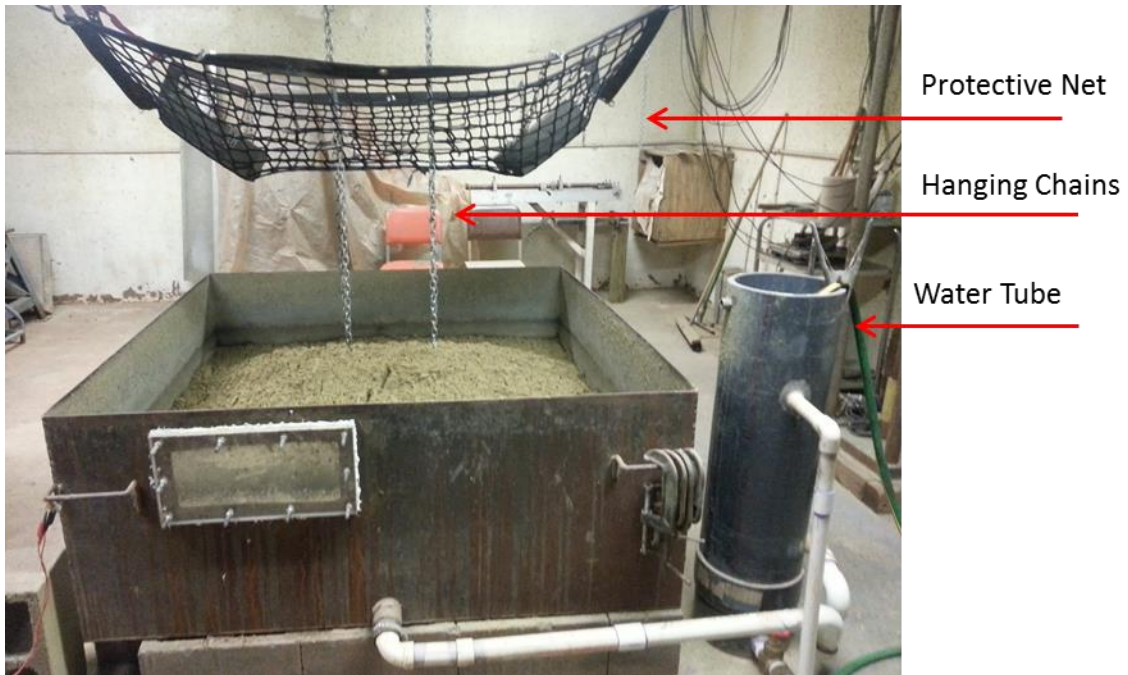
Figure 2.8: Blast tank used for explosive testing
