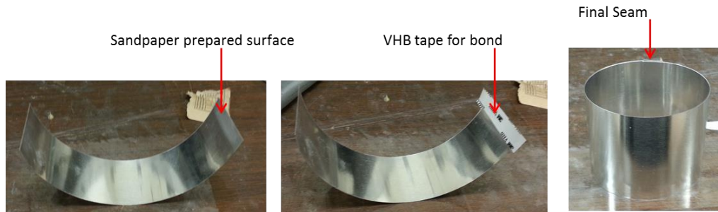
Figure 4.26: Process of creating thin-walled cylinder from shim stock
