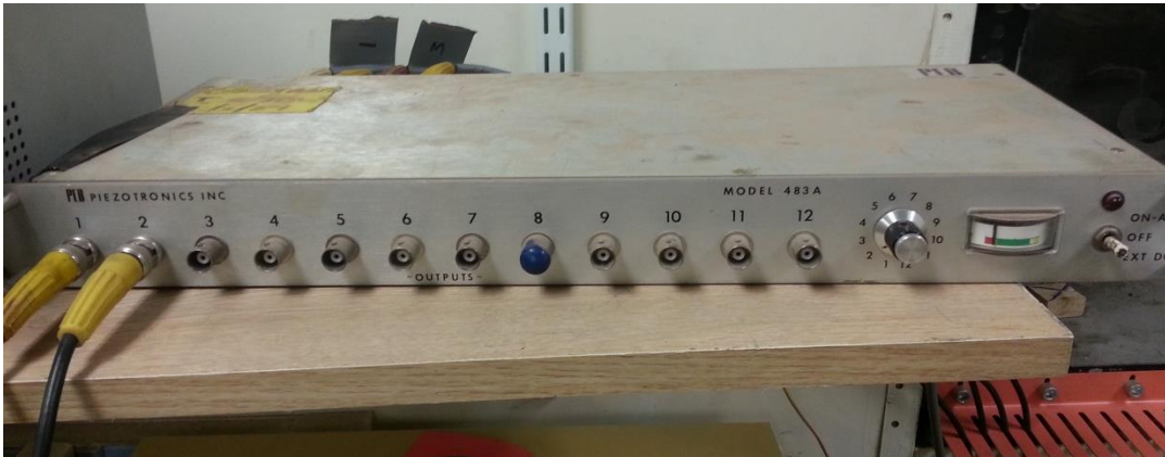
Figure 2.2: Front of the PCB signal conditioner
