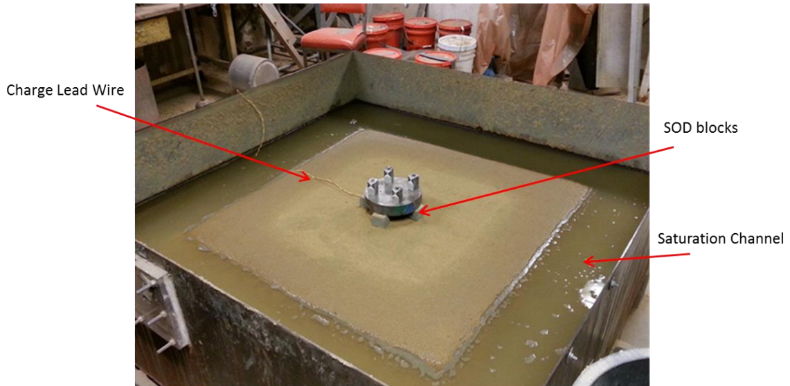
Figure 2.14: Fully prepared blast test sand bed
