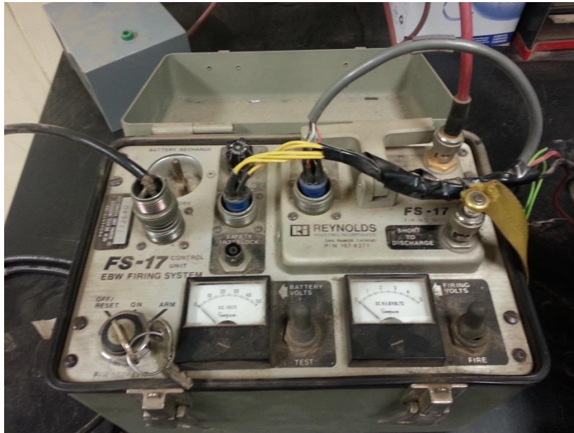
Figure 2.7: FS-17 Firing Module by Reynolds Industries Inc.
