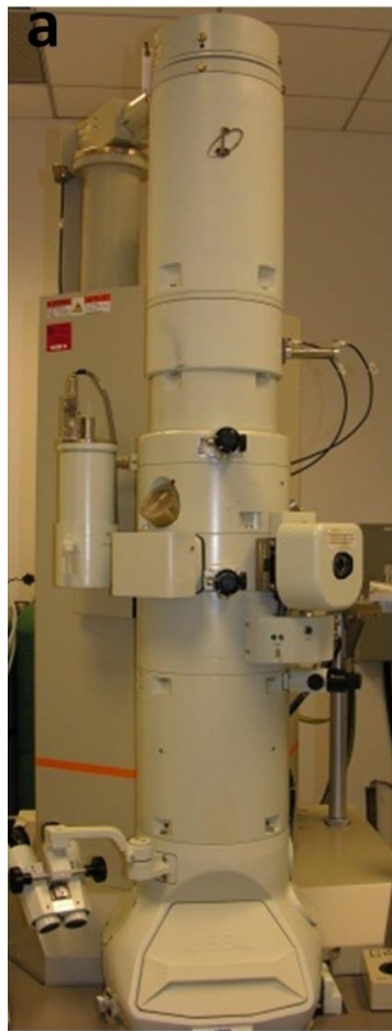
Figure 2.1: (a) A JEOL LaB 6 TEM. (b) A schematic representation of electron optics in TEM. Figure (b) adapted from Ref. [42].
