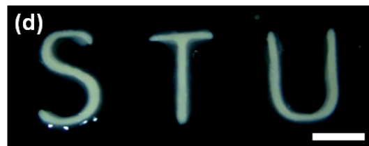
Figure 3.6. (a) Schematic depiction of alginate photopatterning. The photogellable alginate sample is spread as a thin film and UV-irradiated through a mask. After rinsing, gelled regions corresponding to the pattern in the mask are revealed. (b) Alginate gel patterned as an array of ~ 900 mm dots using a steel photomask. Scale bar is 3 mm. (c), (d) Alginate gel patterned as adjacent letters of the alphabet using a stencil. Scale bars represent 5 mm.
