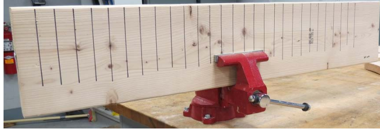
Figure 3. Reciprocating saw cutting wood setup in vice with markings
