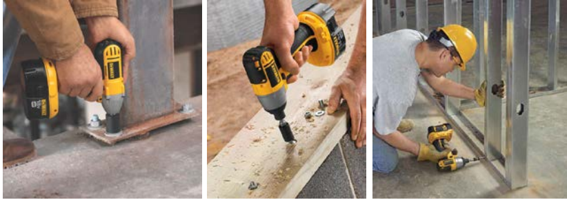
Figure 11. Typical usage of impact driver (Left: Bolt tightening, Middle: Deck fastening, Right: Drill hole) [16]
