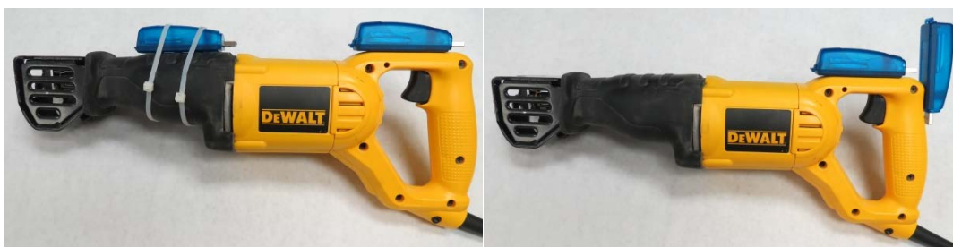
Figure 6. Accelerometer Mounting Position Test Setup (Left: Boot vs. Handle, Right: Horizontal vs. Vertical on Handle)
