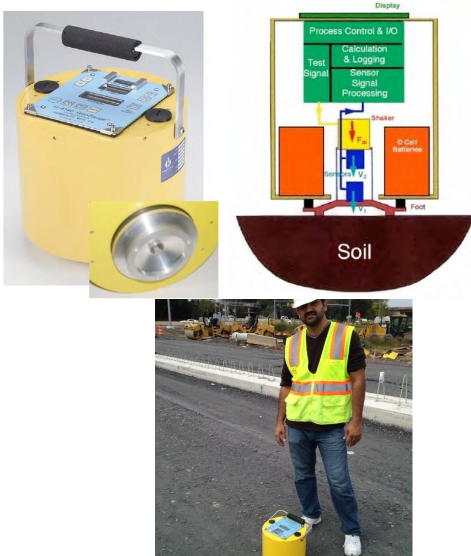
FIGURE B.5: Geogauge used in field testing (After Humboldt Mfg.Co)
