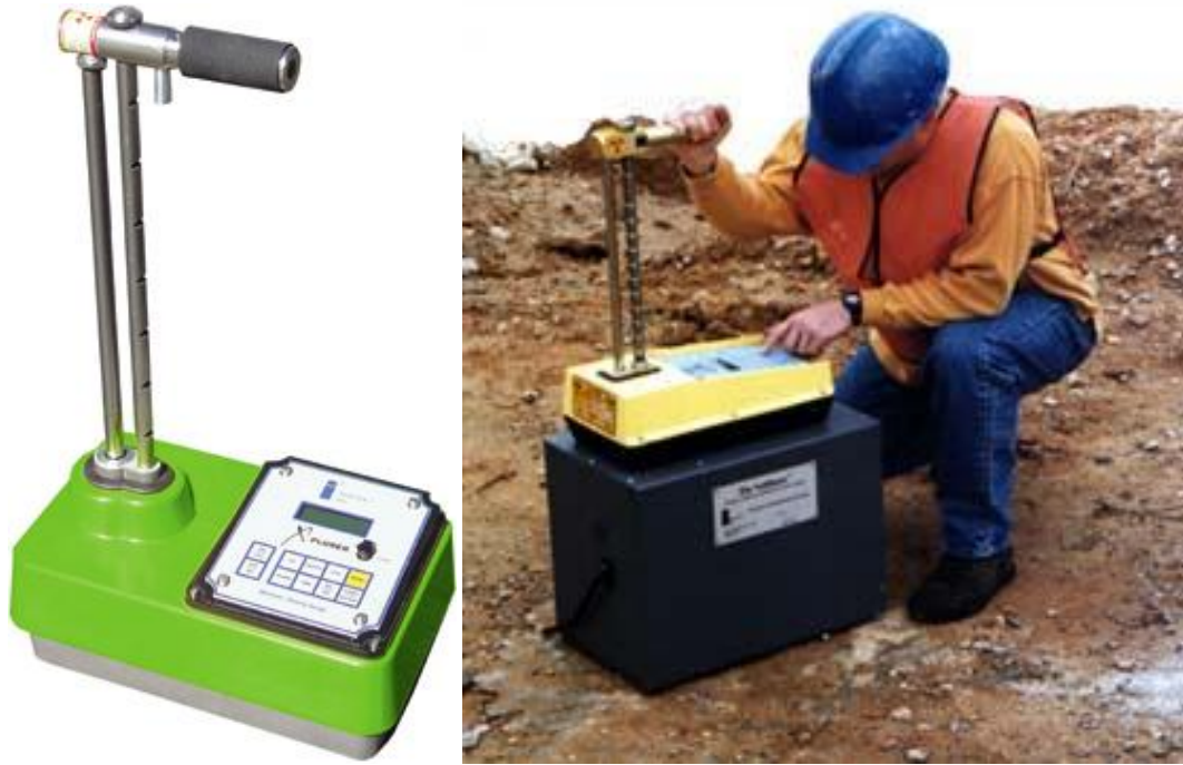
FIGURE B.3: Nuclear density gauge for compaction and moisture content testing.
