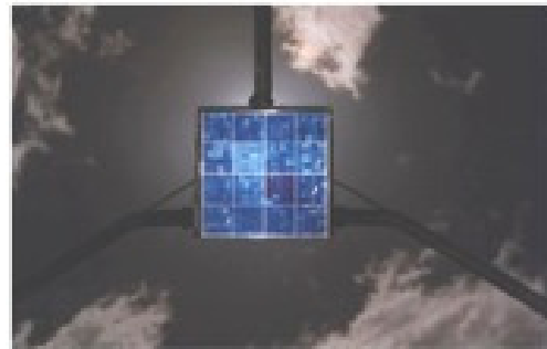
Figure 1.5: Solar Systems' densely packed array visible in its parabolic dish CPV receiver
