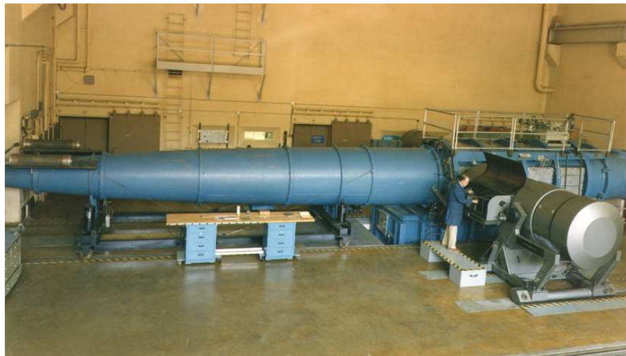
Figure 2.4: Tunnel 9 test section.
