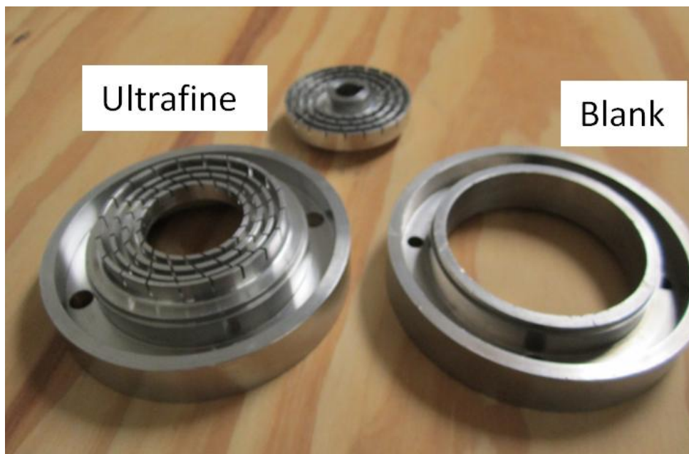
Figure 8.2.1-6: Blank stage as compared to an ultrafine stage.
