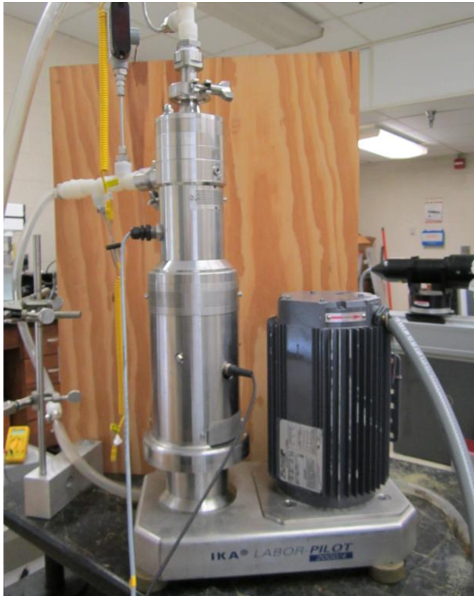
Figure 8.2.2-2: IKA Labor Pilot 2000/4 in-line mixer with Futek TRS600 torque meter installed in-line with the rotor shaft.
