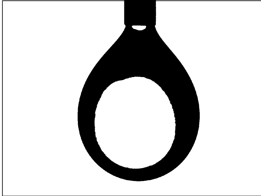
Figure 2.3.6-3: Thresholded pendant drop image using straightforward thresholding.
