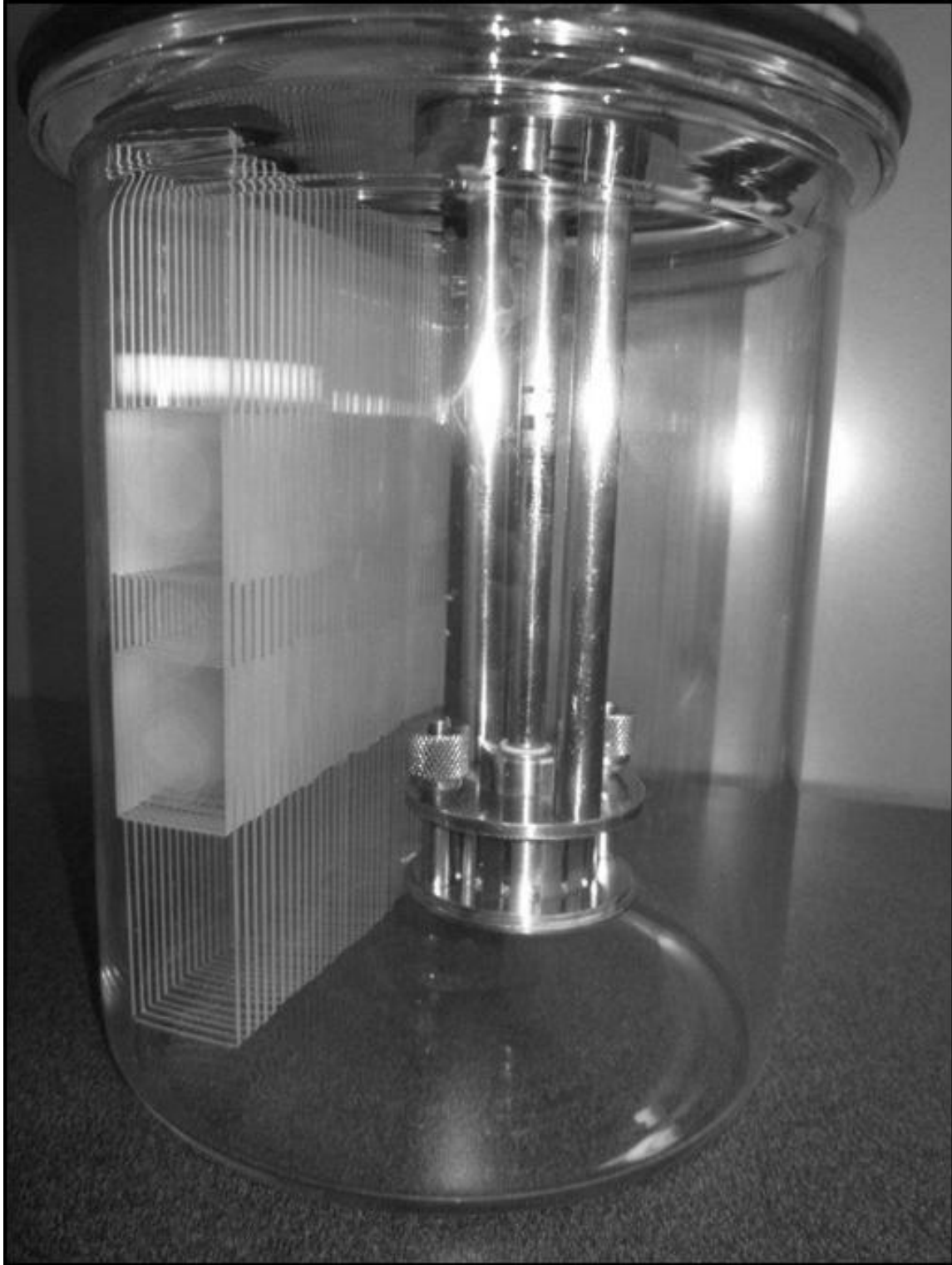
Figure 7.5-1: “Radiator” apparatus. The large amount of hydrophilic surface area provided by gluing microscope slides together in such a fashion should serve to maximize any possible drop adherence to low shear surfaces.
