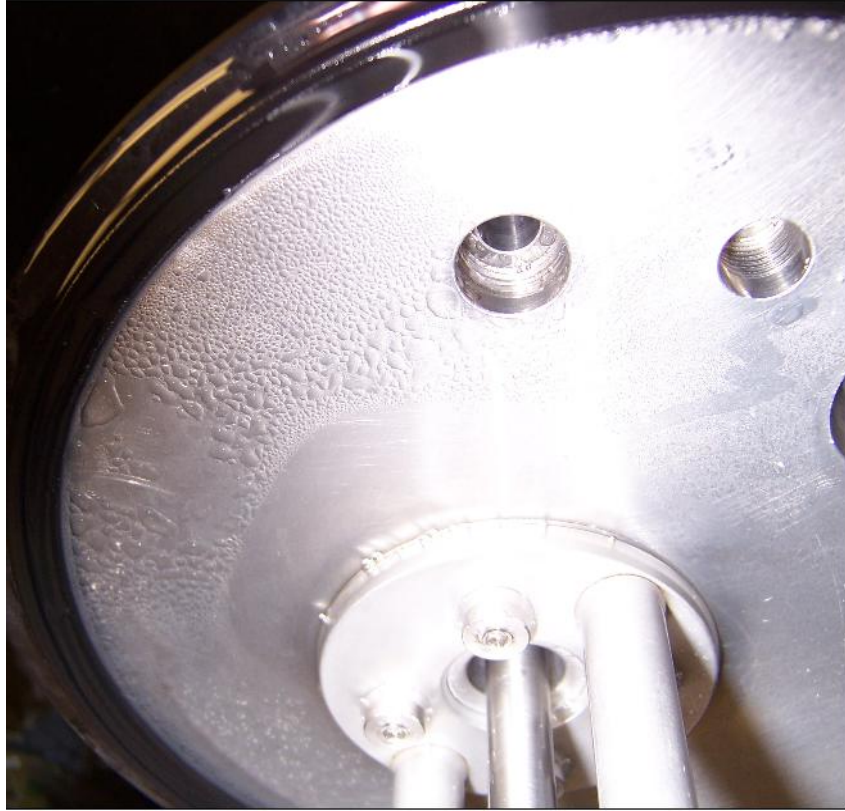
Figure 4.3.2-5: Drops sticking to the underside of the mixer lid. This figure shows that the hydrophobic treatment alone was insufficient to solve the drop sticking problem.
