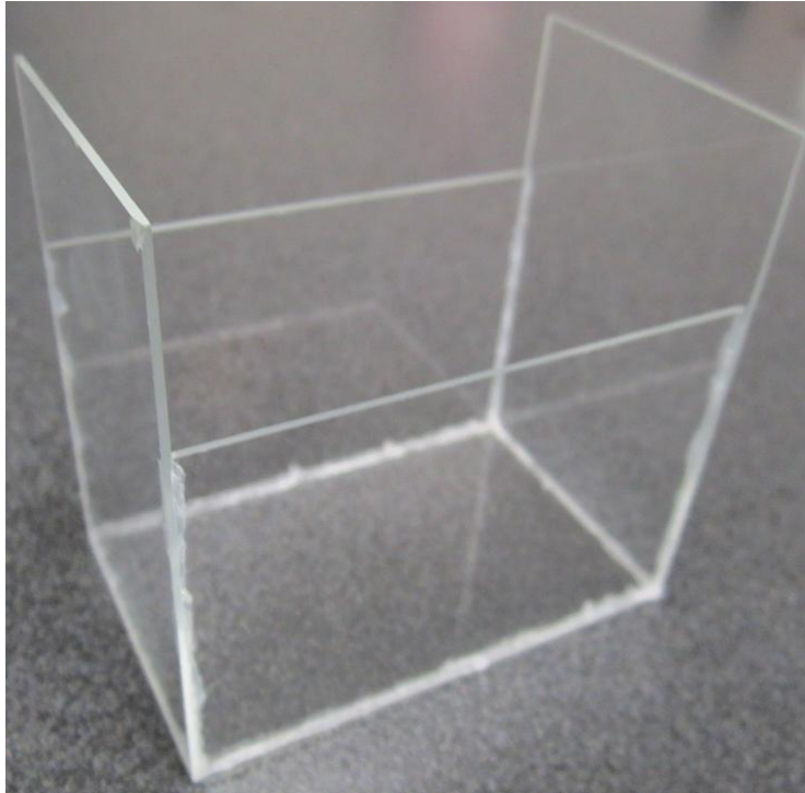
Figure 2.3.6-1: Glass cuvette constructed out of 2" x 3" microscope slides. Used to contain the surrounding phase in liquid-liquid pendant drop experiments to measure interfacial tension.
