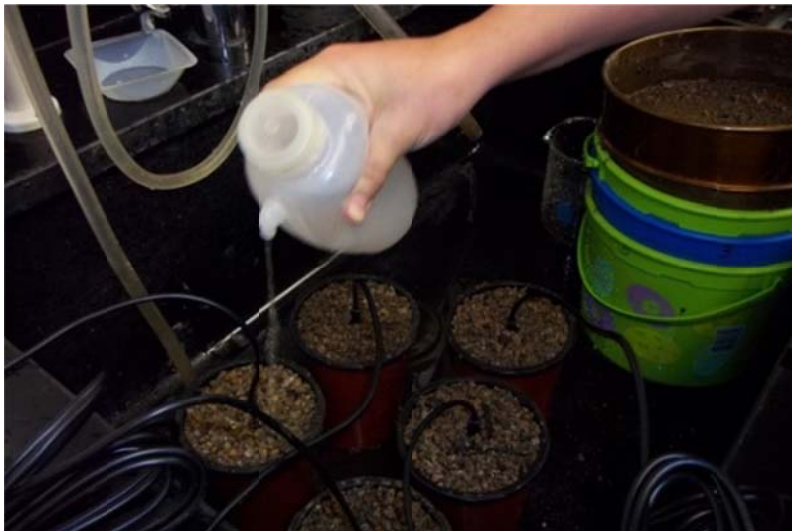
Figure 0.1 Preparing the greenroof substrate for calibration
