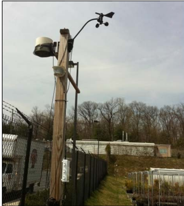
Figure 3.3 The decagon weather station included a rain gauge, pyranometer, PAR sensor, Davis-cup anemometer, and a relative humidity sensor.
