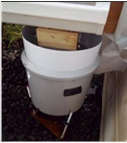
Figure 3.2 One of the 40mL tipping bucket rain gauges for collecting platform runoff, installed in May of 2011
