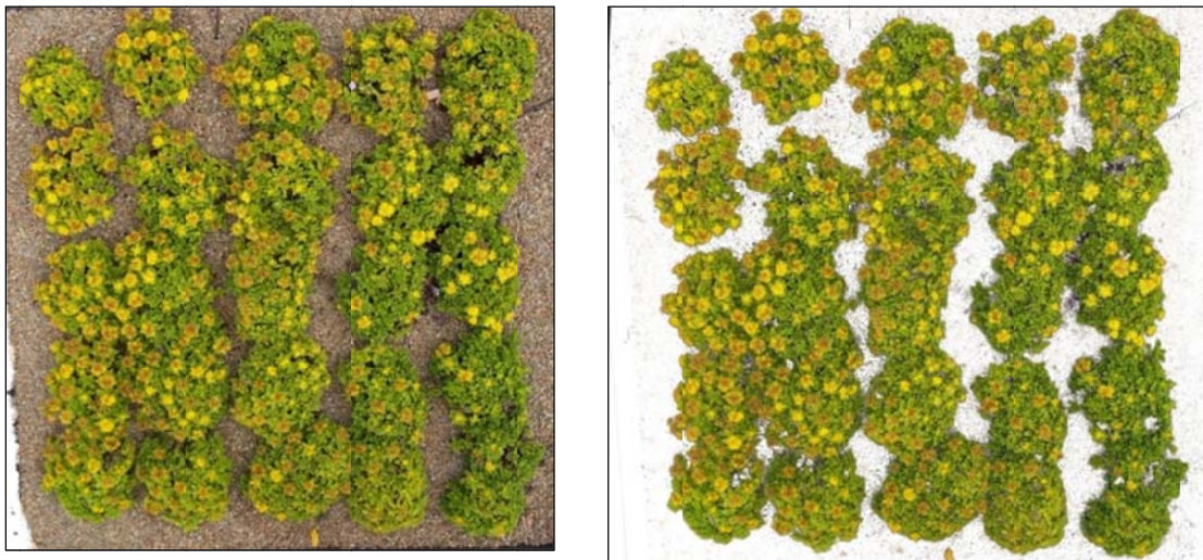
Figure 3.4 Example coverage analysis. The number of pixels in the picture on the right would be divided by the number of pixels in the picture on the left. In this example, a platform planted in S. kamtschaticum is shown from the spring of 2012; 69.2% coverage was estimated.
