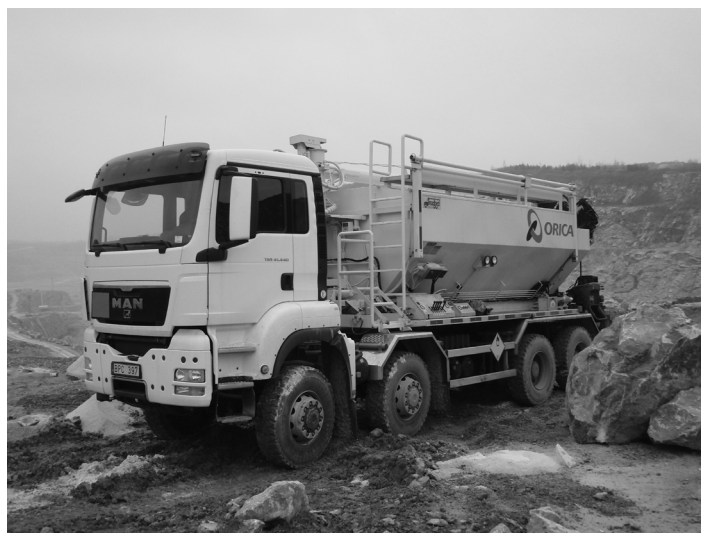
Figure 11.4: Self-propelled unit with mixer-loading equipment.
