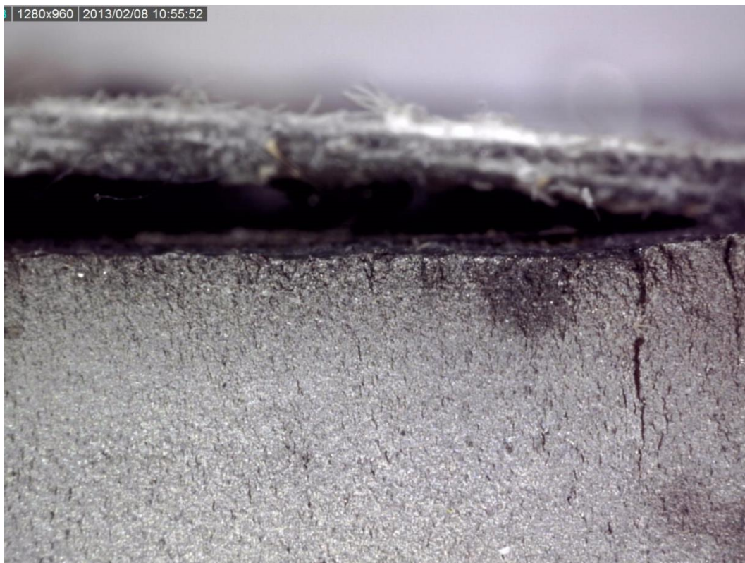
Figure 4.29. Pictures of crack propagation zones on the fracture surface of specimen WTJ5 (magnification factor for microscopic image labeled 1, 2, 3 = 65): (a), (b)
