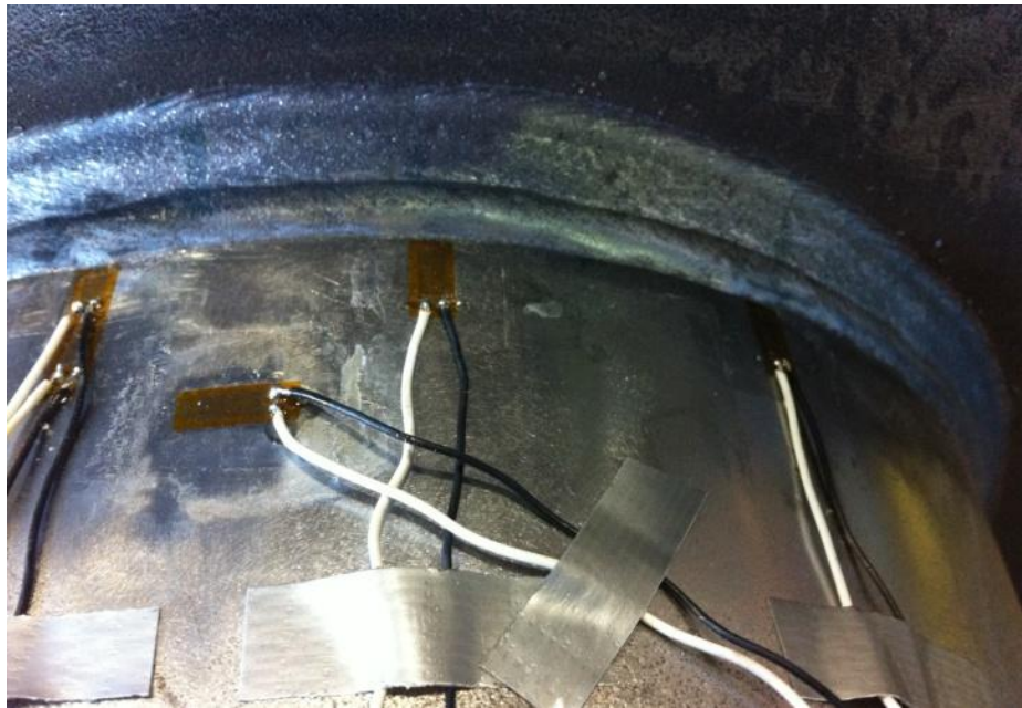
Figure 4.5. View of strain gauges on specimen
