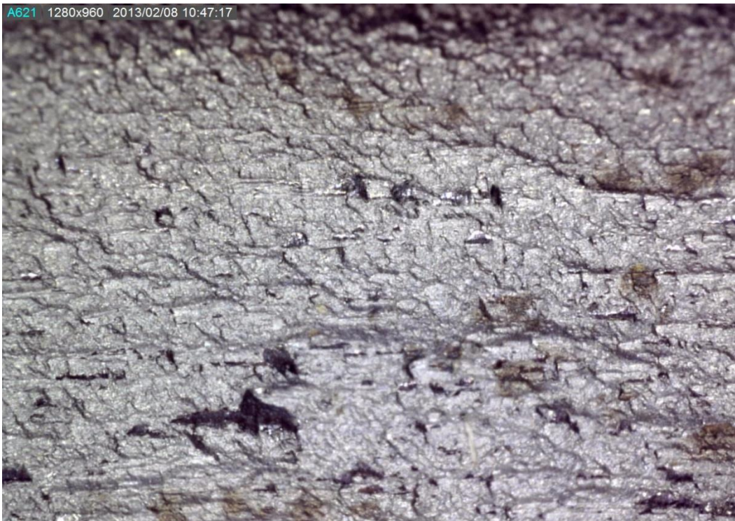
Figure 4.26. Pictures of crack propagation zones on the fracture surface of specimen WTJ1 (magnification factor for microscopic image labeled 1, 2, 3 = 65): (c), (d)
