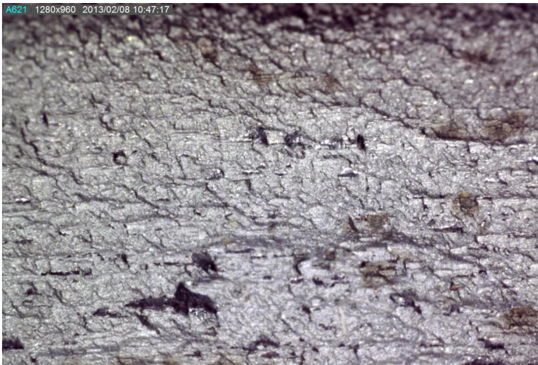
Figure 4.28. Pictures of crack propagation zones on the fracture surface of specimen WTJ4 (magnification factor for microscopic image labeled 1, 2, 3 = 65): (c), (d)
