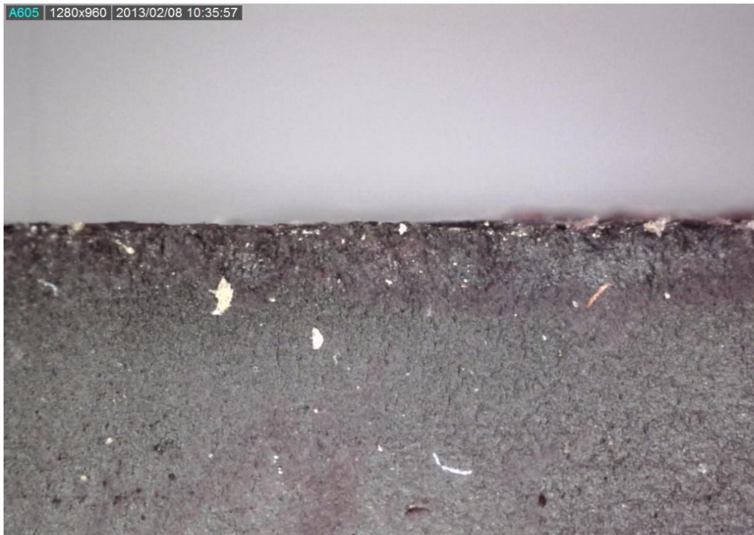
Figure 4.25. Pictures of crack propagation zones on the fracture surface of specimen WTJ1 (magnification factor for microscopic image labeled 1, 2, 3 = 65): (a), (b)
