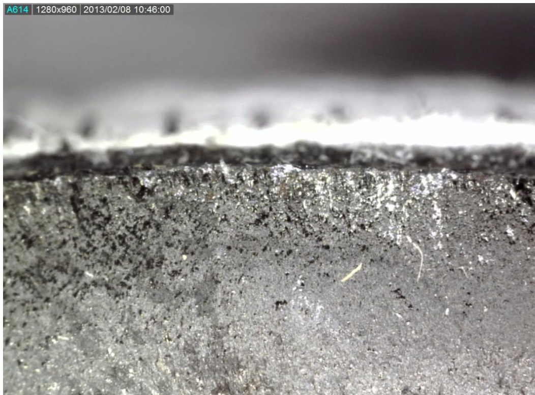
Figure 4.27. Pictures of crack propagation zones on the fracture surface of specimen WTJ4 (magnification factor for microscopic image labeled 1, 2, 3 = 65): (a), (b)
