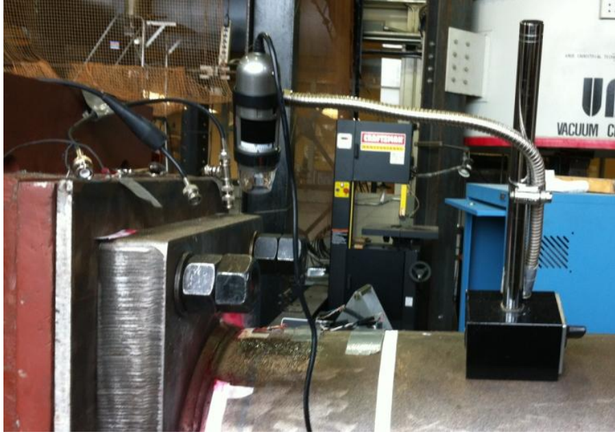
Figure 4.6. Measuring crack size using digital microscope
