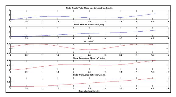
Figure 5.14: Blade Section Twist and Bending With Arbitrary Loading
