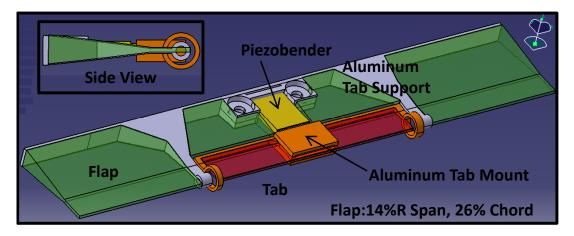
Figure 1.26: Airfoil Schematic of Flap+Tab System
