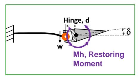
Figure 2.8: Flap Driven by Piezobender Schematic
