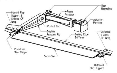
Figure 1.18: Hall and Prechtl Flap Mechanism
