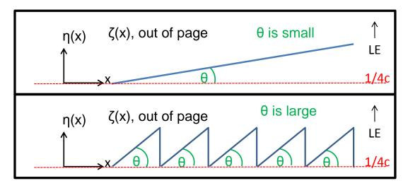
Figure 5.11: Sawtooth Pattern Required for Sufficiently Large Sensor  $\theta$
