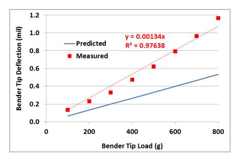
Figure 2.22: 12-Layer PZT-5K4 Bender Stiffness - Poor Bond
