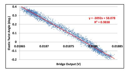
Figure 5.21: Calibration Curve for Single Twist Sensor
