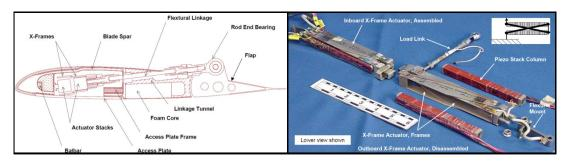
Figure 1.19: SMART rotor flap schematic and 2X-Frame
