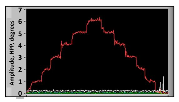
Figure 4.1: Outboard Flap Amplitude Closed-Loop Control at 900 RPM
