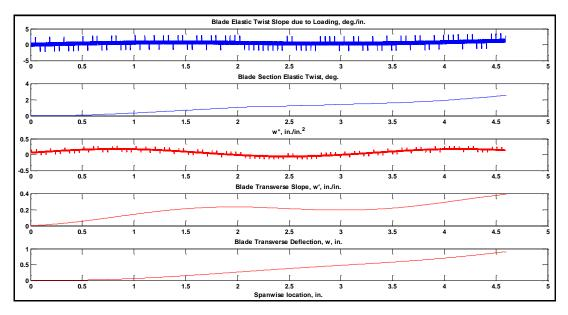
Figure 5.17: Blade Section Twist and Bending With Arbitrary Loading, Noise, Local Discontinuities
