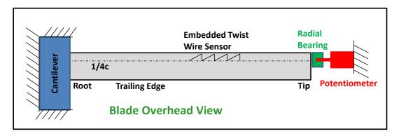
Figure 5.20: Single Point Experimental Setup
