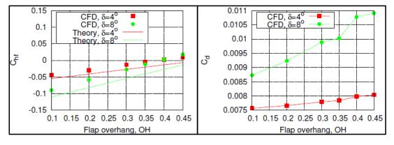
Figure 3.7: Effect of Overhang: Left: Flap Hinge Moment, Right: Drag [82]
