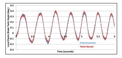
Figure 5.22: Comparison of Single Twist Sensor to Actual
