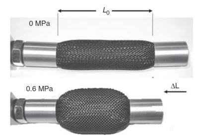
Figure 1.32: PAM at no pressure and contracted
