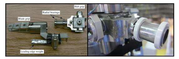
Figure 3.29: Left: Steel Radial Ball Bearings, Right: Replaced by all Ceramic Bearings
