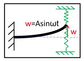
Figure 2.43: 4-Layer Bender Constrained by Spring
