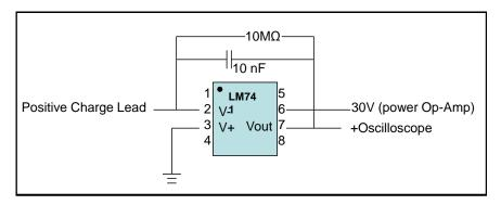
Figure 2.25: Schematic for Charge Amplifier Circuit
