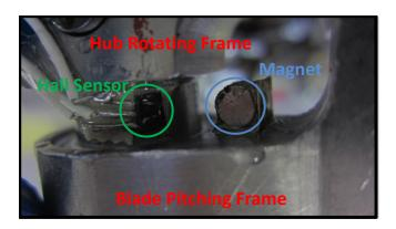
Figure 3.30: Hall Sensor for Measuring Blade Root Pitching
