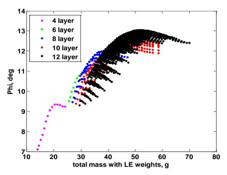
Figure 2.12: Flap Angle vs. Total Mass including LE Weight Required ramic layers.
