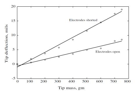
Figure 2.20: Bender Stiffness: Effect of electrical boundary conditions
