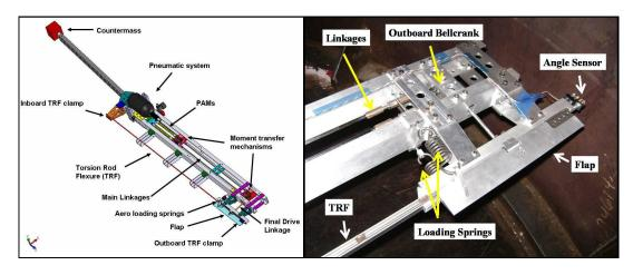
Figure 1.34: PAM flap system for vacuum chamber
