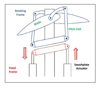
Figure 1.1: Swashplate Diagram
