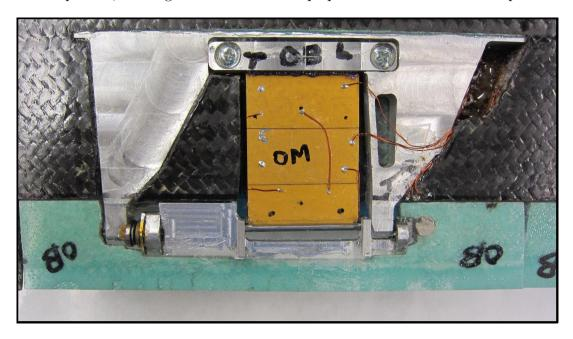
Figure 3.23: Flap Assembly in Blade Close-Up
