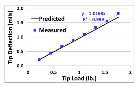
Figure 2.24: 12-Layer PZT-5K4 Bender Stiffness - Good Bond
