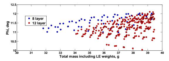
Figure 2.14: Bender Optimization: 8 vs. 12 Layers, Flap Angle vs. Total Mass
