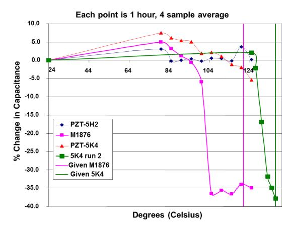
Figure 2.16: Curie Temperature Measurement
