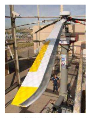
Figure 1.20: SMART rotor hoverstand testing
