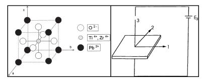
Figure 1.16: Left: Piezoelectric Crystal Molecule, Right: Piezoplate
