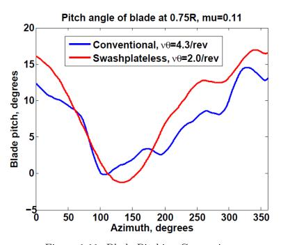
Figure 1.11: Blade Pitching Comparison
