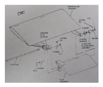
Figure 1.14: KMAX Servo Flap Exploded View [28]
