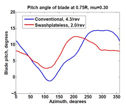
Figure 1.12: Blade Pitching Comparison
