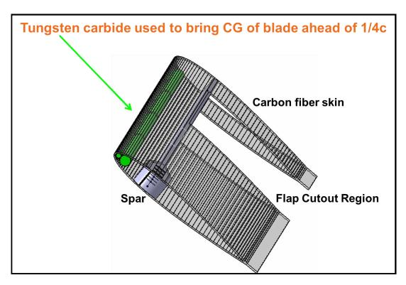
Figure 3.2: Main Blade Components
