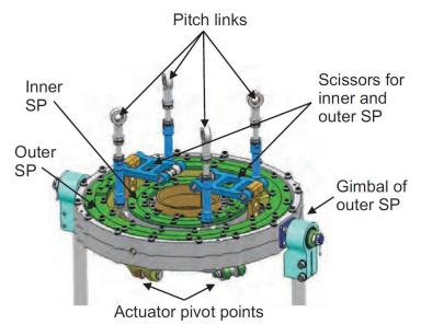
Figure 1.4: Multiple Swashplate (SP) Mechanism
