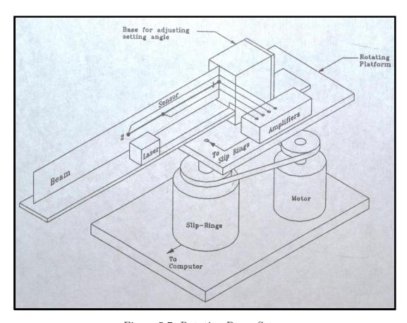
Figure 5.7: Rotating Beam Setup
