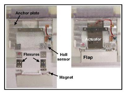
Figure 3.9: Roget TE Flap Setup
