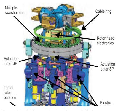
Figure 1.5: META mechanism diagram including actuators
