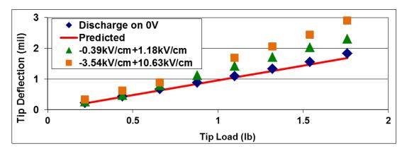
Figure 2.31: 12-Layer PZT-5K4 Bender Compliance for 2Hz Field
