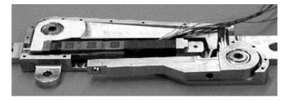
Figure 1.17: L-L mechanism for stack actuator stroke amplification [37]
