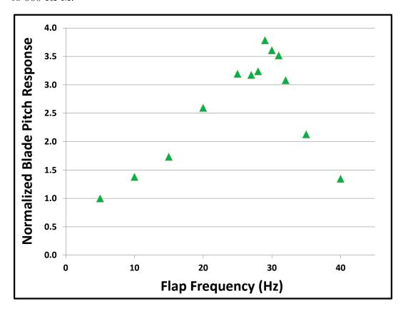
Figure 3.31: Blade Pitch Frequency Response to TE Flaps with Ceramic Bearings, 900 RPM
