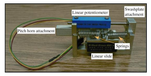
Figure 3.27: Initial Soft Pitch Link
