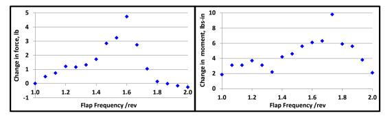
Figure 4.9: Hub Force and Moment at 900 RPM due to TE Flaps
