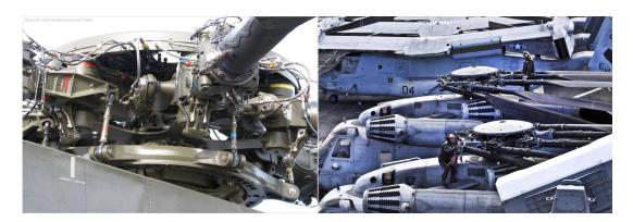
Figure 1.2: CH-53 Rotor Swashplate
