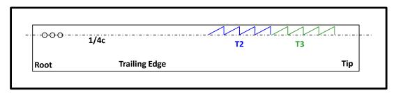
Figure 5.12: Twist Sensors in Mach Scale Blade Skin
