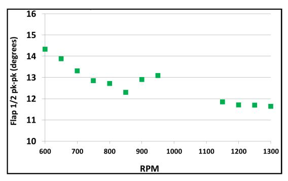
Figure 3.20: Single OB Flap with Overhang, Thrust+Radial Bearings in Vacuum, 38.3 Hz Flap Amplitude driven at -50V/+150V
