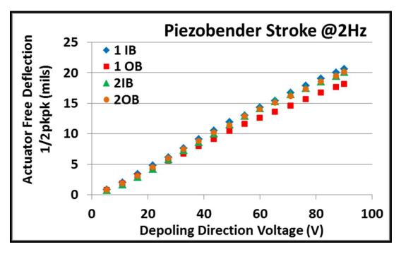
Figure 3.24: Maximum Bender Strokes at 2 Hz
