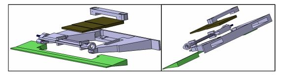
Figure 3.4: Flap Assembly Exploded View
