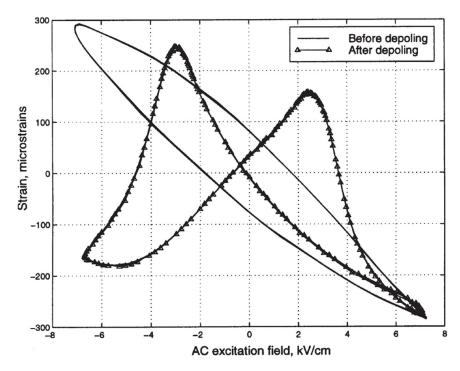
Figure 2.4: Piezoceramic plate, PZT-5H2, Free Strain-Electric Field Loops [35]
