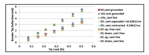
Figure 2.40: 4-Layer Bender Stiffness with Various Cantilever Electrical Fields
