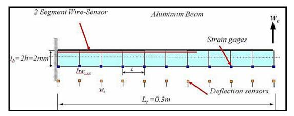
Figure 5.5: Distributed Wire Sensor in Cantilever Beam
