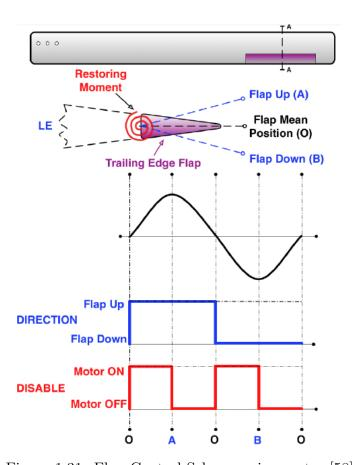
Figure 1.31: Flap Control Scheme using motor [58]
