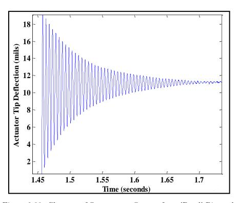
Figure 2.38: Close-up of Squarewave Output from 'Dead' Bimorph
