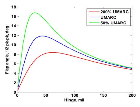
Figure 2.9: Effect of Hinge Distance on Flap Amplitude
