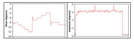
Figure 4.2: Outboard Flap Mean Closed-Loop Control at 900RPM, Constant Amplitude
