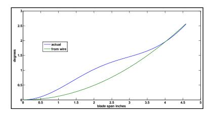
Figure 5.16: Blade Section Twist: Actual vs. Sensor With Arbitrary Loading
