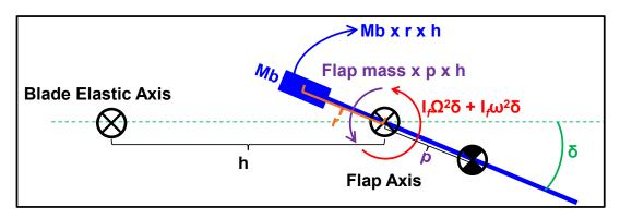
Figure 3.5: Flap Free Body Diagram
