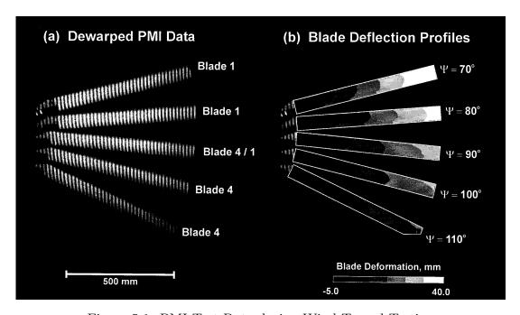
Figure 5.1: PMI Test Data during Wind Tunnel Testing
