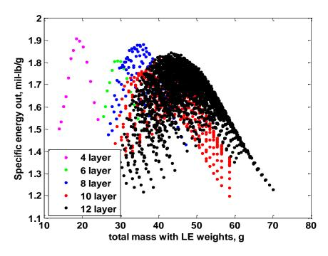
Figure 2.11: Bender Specific Energy vs. Total Mass including LE Weight Required
