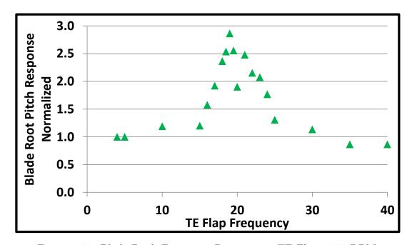
Figure 3.28: Blade Pitch Frequency Response to TE Flaps, 900 RPM
