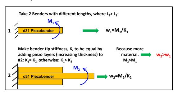
Figure 2.6: Effect of Length Conceptualization
