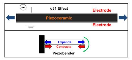
Figure 2.2: Top: Single layer, Bottom: Piezobender Bimorph
