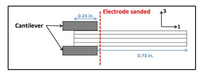
Figure 2.39: 4-Layer Bender Stiffness with Electrically Separate Cantilever
