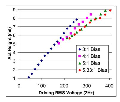
Figure 2.29: Effect of increasing bias on PZT-5K4 Bender Stroke
