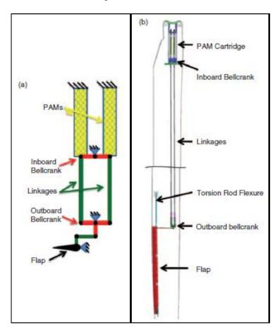
Figure 1.33: a) PAM Cartridge schematic and b.) Blade Flap Schematic [59]
