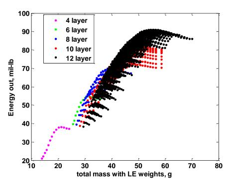
Figure 2.10: Bender Energy vs. Total Mass including LE Weight Required
