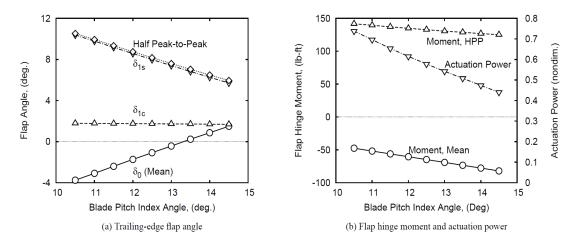
Figure 1.6: Effect of Index Angle on flap control angles, actuation power and moment, Flap overhang of 0.05c and  $\mu = 0.32$  [26]
