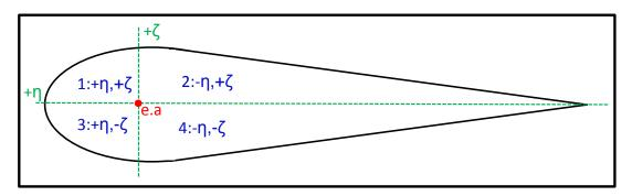
Figure 5.10: Blade Profile Split into Quadrants for Measuring Twist
