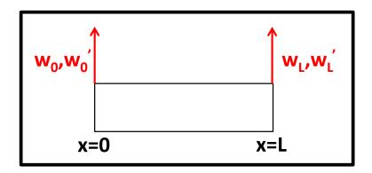
Figure 5.4: Beam Finite Element
