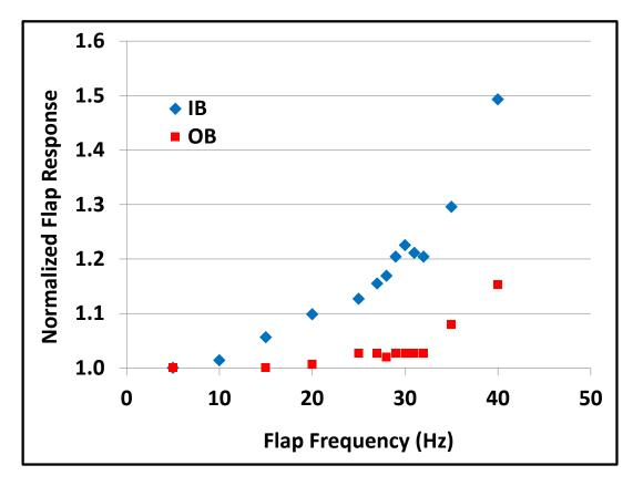
Figure 3.26: Blade 1 Flap Freq Sweep at 900RPM - Fixed Driving Voltage Normalized at 2Hz
