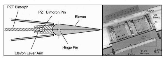
Figure 1.22: Fulton's Blade schematic and exploded view picture
