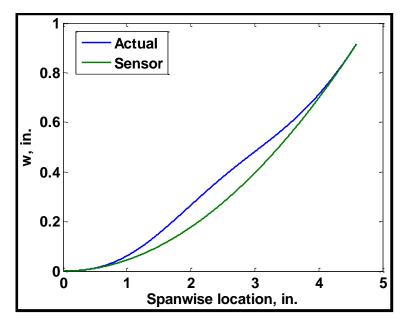
Figure 5.18: Blade Section Bending: Actual vs. Sensor With Arbitrary Loading, Noise, Local Discontinuities
