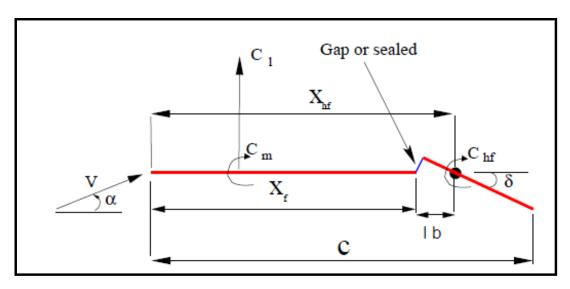
Figure 3.6: Flap with Overhang Schematic
