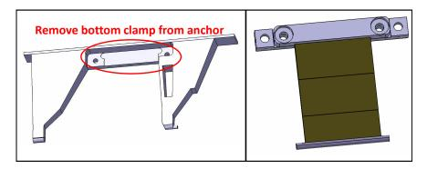
Figure 6.3: Modification to allow for flap mean and hinge adjustment for primary control implementation
