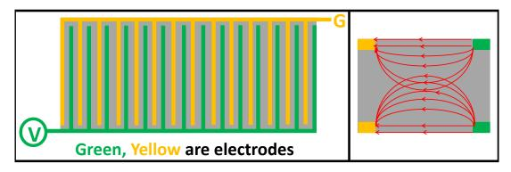
Figure 6.1: a) Top view of piezoplate with interdigitated electrodes b) Electric field lines between IDEs
