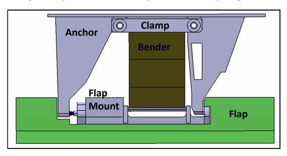
Figure 3.3: Flap Assembly Exploded View
