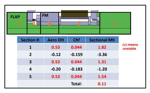
Figure 3.15: Flap Aerodynamic Stiffness
