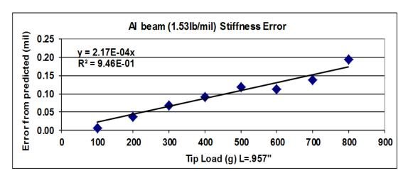
Figure 2.19: Best Case Cantilever Stiffness
