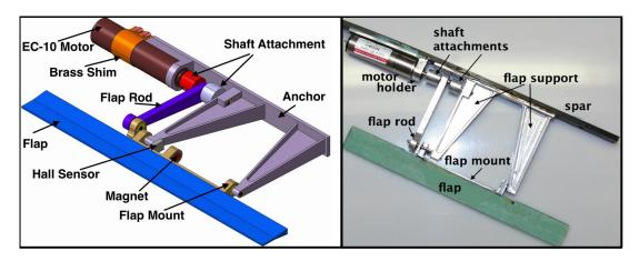
Figure 1.29: Brushless DC motor-flap schematic and picture [58]
