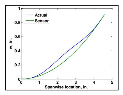
Figure 5.15: Blade Section Bending: Actual vs. Sensor With Arbitrary Loading
