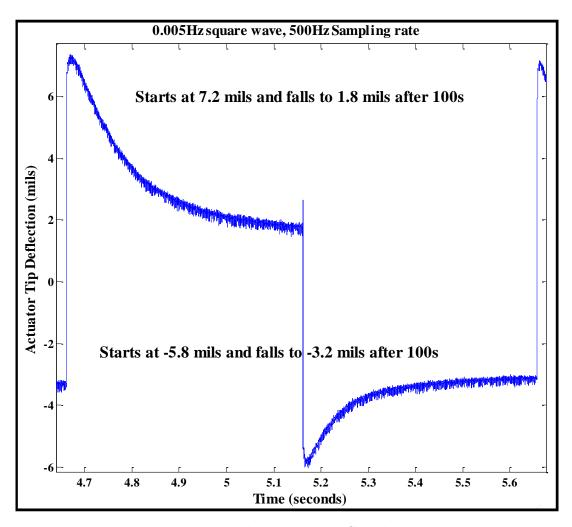
Figure 2.42: 4-Layer Bender with Dead Cantilever Response to  $-3.54 \rm kV/cm/+10.63 kV/cm~0.005 Hz$  Squarewave
