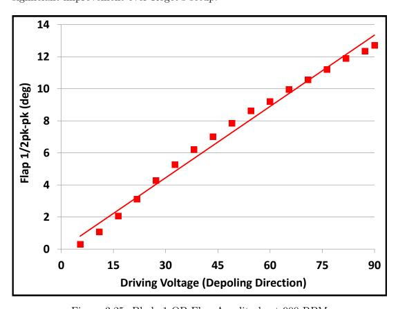
Figure 3.25: Blade 1 OB Flap Amplitude at 900 RPM
