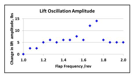
Figure 4.8: Lift Oscillation at 900 RPM due to TE Flaps
