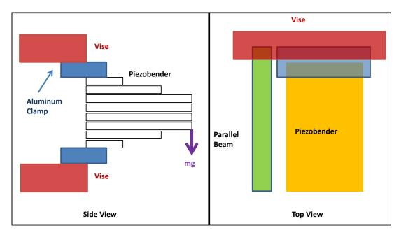
Figure 2.17: Measuring Bender Stiffness with Parallel Beam
