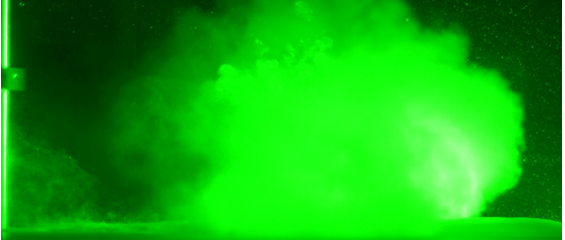
Figure 3.15: Dual-phase flow visualization with the rotor operating at 450rpm ( Re_{\text{tip}} = 5.98 \times 10^4 ).
