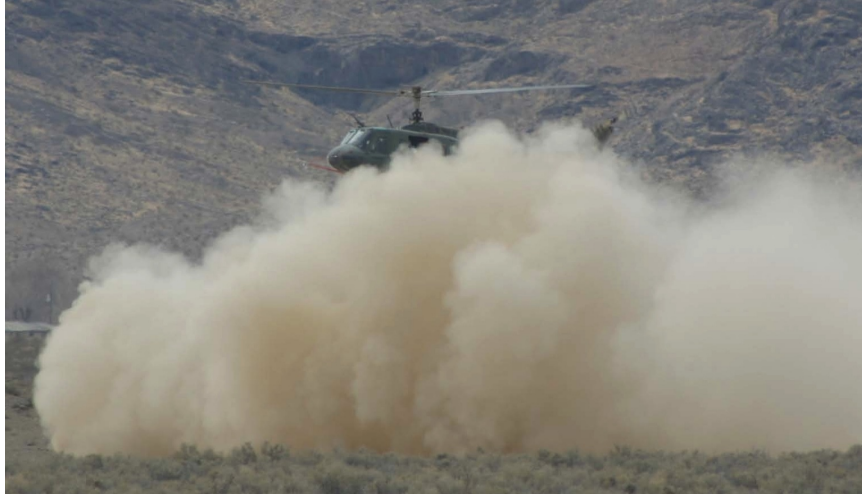
Figure 1.1: Brownout as experienced by a helicopter landing in a desert environment. (Courtesy of Optical Air Data Systems LLC.)
