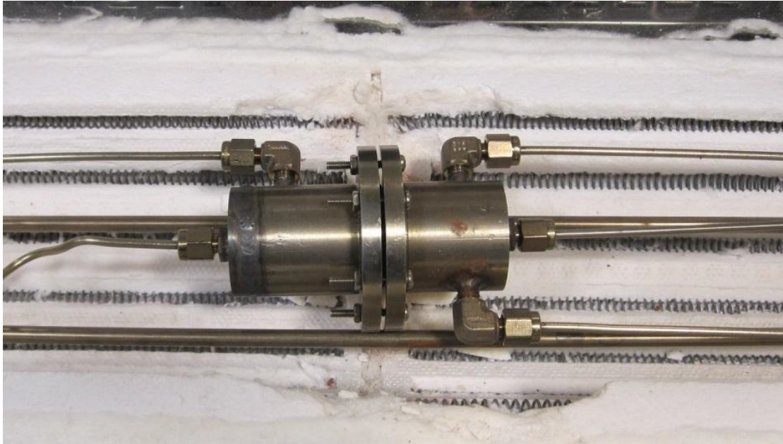
Figure 3-7. Membrane housing mounted inside Carbolite furnace.
