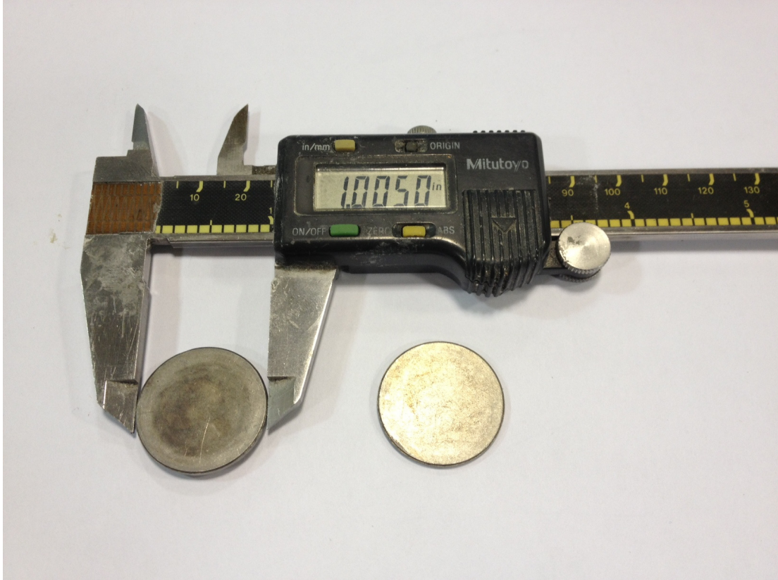
Figure 3-1. Photograph of palladium (left) and palladium-copper (right) membrane.
