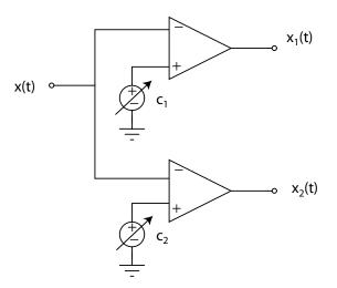
Figure 5.2: Diagram of circuit for generating binary sequences.
