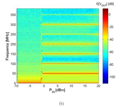
Figure 2.11: (a) Time evolution of output signal when input RF signal has power of 14 dBm and frequency of 100 MHz (b) Spectrogram of output voltage as input RF power is varied. Only the superharmonics are observed.
