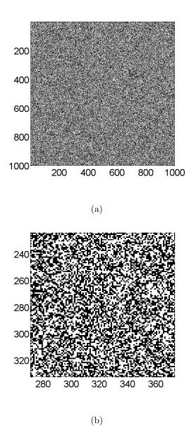
Figure 5.5: (a) Grayscale plot for output bit sequence after converting to square matrix. (b) Inset of (a). Black pixels represent 1, and white pixels respresent 0.
