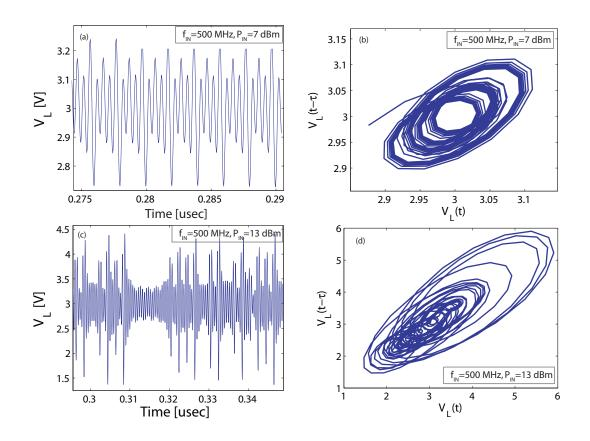
Figure 3.10: (a) Time evolutions of load voltage  $V_L$  (b) Delay phase space diagram, when the circuit is excited by the input RF signals with the frequency of 500MHz and RF power of 7 dBm. (c) Time evolutions of load voltage  $V_L$  (d) Delay phase space diagram, when the circuit is excited by the input RF signals with the frequency of 500MHz and RF power of 13 dBm.
