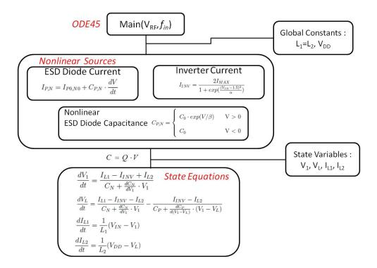
Figure 3.9: Flowchart for numerical modeling. The system of ODE is solved using 4th order Runge-Kutta method with the nonlinear source listed, such as nonlinear diode equations, nonlinear transconductance of the inverter, and nonlinear ESD diode capacitance.
