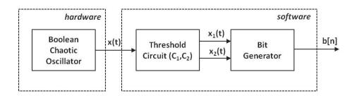
Figure 5.1: Schematic diagram of random number generation using CMOS boolean chaotic oscillator.
