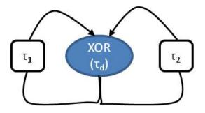
Figure 4.1: Example of Boolean Chaos. Two delays  $(\tau_1 \text{ and } \tau_2)$  are inputs of XOR with response time  $(\tau_d)$ .
