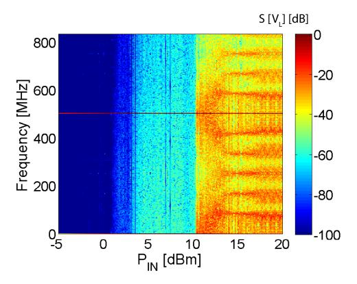
Figure 3.11: Numerical results of spectrogram of load voltage, when the circuit is excited by input RF signal with a frequency of 500 MHz as RF power is varied.
