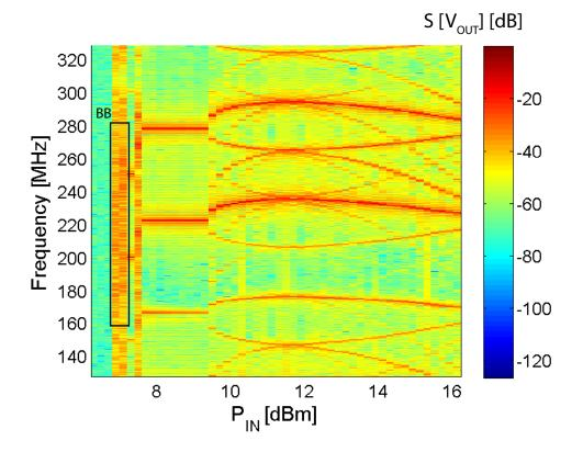
Figure 2.13: Evidence of chaotic oscillation such as complex spectrum and broadband spectrum (BB).
