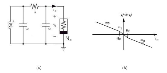
Figure 1.2: (a) Circuit diagram of Chua chaotic circuit. (b) Current-voltage transfer characteristics of Chua diode [19].
