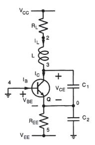
Figure 1.5: Circuit diagram of a bipolar junction transistor Colpitts oscillator [24].
