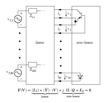
Figure 3.3: Schematic diagram explaining how the harmonic balance simulation operates. F(V) solves the nonlinear and linear parts separately. Y is the transadmittance matrix for the linear parts, and Q and  $I_G$  are the frequency-domain factors for the nonlinear circuits.
