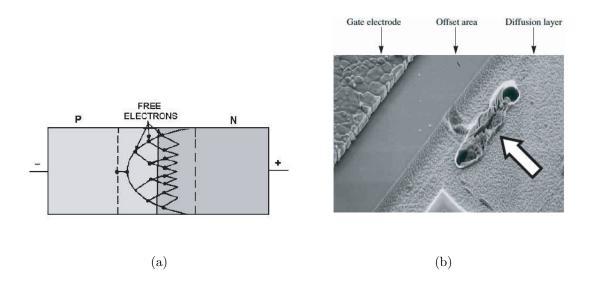
Figure 1.8: (a) Diagram of PN-junction in the Avalanche breakdown. High reverse field creates the multiplications of free electrons by impact ionizations. (b) Scanning electron microscopy image of a junction breakdown. The arrow region shows a physical PN-junction damage.
