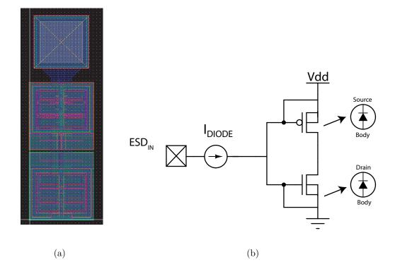
Figure 2.8: (a) Layout of ESD protection circuits. The topmost square represents a pad design, and the two bottom squares represent several ESD MOSFETs, connected as back-to-back diode. (b) ESD event occurring at the input of CMOS digital circuits.  $V_{DD}$  is biased at 4V, and  $I_{DIODE}$  is measured at the input.
