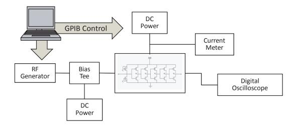
Figure 2.10: Experimental setup for measuring output voltage, supply current, and input rectified voltage. RF signal is directly injected at the input of device-under-test (DUT), mounted on the PCB, with varying RF power and frequency. The digital oscilloscope has a high sampling rate to measure the real time input and output voltages, and the DC supply current is measured with a current meter.
