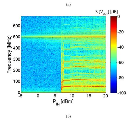
Figure 2.12: (a) Time evolution of output signal when input RF signal has power of 14 dBm and frequency of 500 MHz (b) Spectrogram of output voltage as input RF power is varied.
