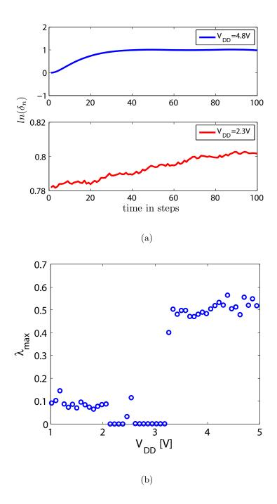
Figure 4.5: (a) Average logarithmic distance between trajectories when  $V_{DD}$  is 4.8V (top) and 2.3V (bottom). Top figure shows a positive slope while the bottom has a slope close to zero. (b) Maximum Lyapunov exponents ( $\lambda_{max}$ ) with varying  $V_{DD}$  as the measured data for each  $V_{DD}$  are calculated for  $\lambda_{max}$ . After  $V_{DD}$  reaches 3.3V, the circuit enters chaotic region, resulting in positive  $\lambda_{max}$ .
