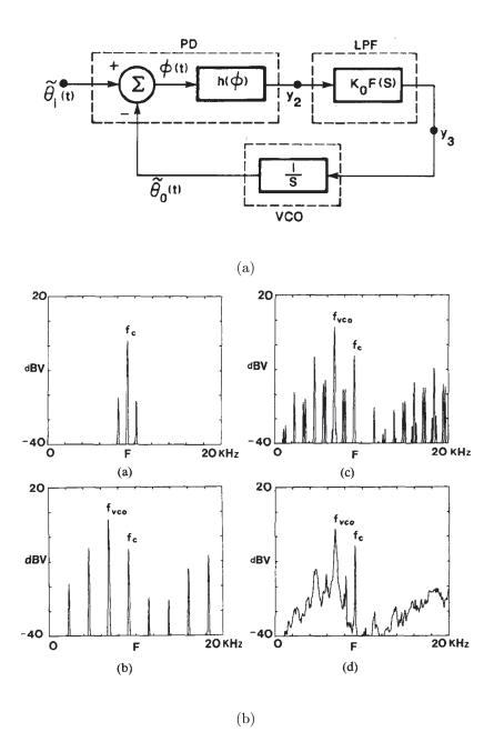
Figure 1.4: (a) Block digram of a phase-lock loop (PLL). (b) The bottom right figure shows a broad chaotic spectrum [23].
