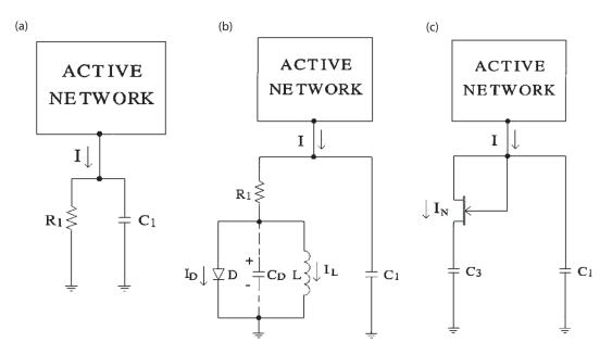
Figure 1.7: Classes of core chaotic oscillators. (a) sinusoidal oscillator with a parallel RC, (b) using diode inductor composite, and (c) with FET and capacitor composite [33].
