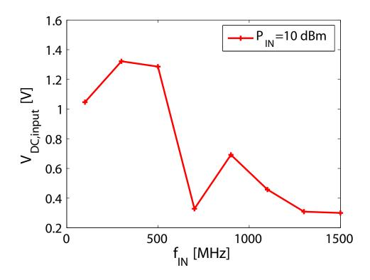
Figure 3.5: DC detected input voltage as frequency of input is changing and RF amplitude is fixed at 10 dBm. The trough around 700 MHz corresponds with the decline of forward transmission coefficient in Fig. 3.4
