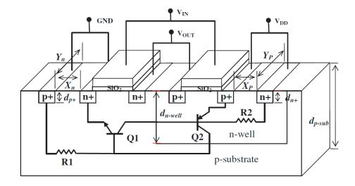
Figure 1.9: Schematic diagram of CMOS inverter showing two parasitic bipolar junction transistors  $Q_1$  and  $Q_2$ . Latch-up effects are due to the BJT action.
