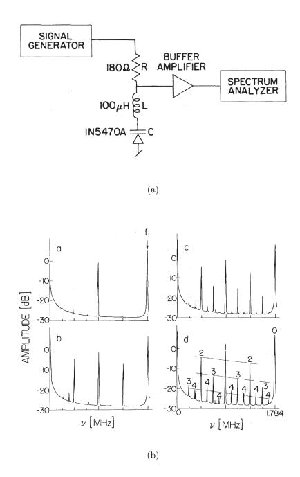
Figure 1.1: (a) Circuit diagram of driven anharmonic oscillator. This circuit consists of a nonlinear capacitor, a resistor, and an inductor [1]. (b) Voltage spectrums as RF amplitudes change, driving circuits from periodic oscillation to chaotic oscillation.
