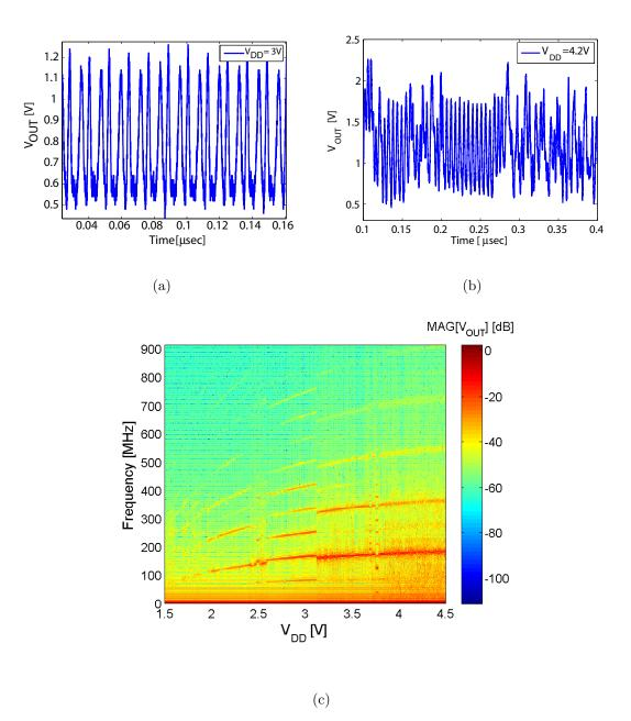
Figure 4.8: (a) Time evolution of periodic oscillation when the circuit is biased at 3V. (b) Time evolution of chaotic oscillation when the circuit is biased at 4.2V. (c) Frequency spectrum of output voltage signal with varying  $V_{DD}$ . Broad spectrum with numerous subharmonics, reaching from DC to 300 MHz, is observed.
