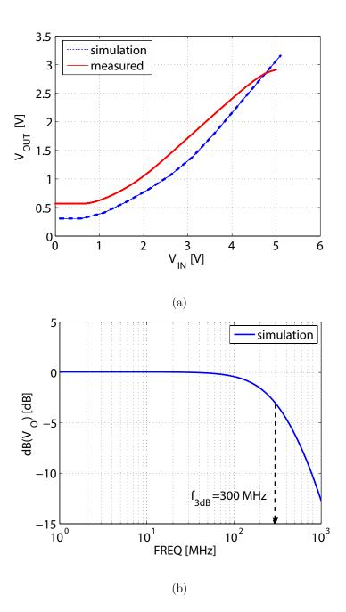
Figure 4.7: (a) Transfer characteristics of the buffer for measurement and simulation. (b) Bode plot of simulated output voltage of buffer. This buffer is capable of 3dB cut-off frequency of 300 MHz and has wide input ranges for unity gain. The cutoff frequency of the buffer is determined from the amount of current flowing through amplifiers and loading capacitance.
