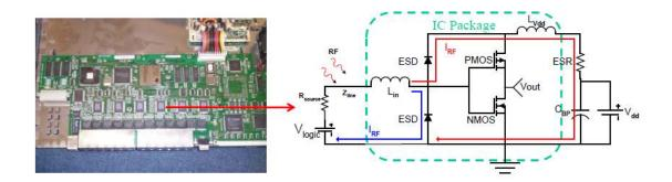
Figure 2.1: Schematic diagram and basic elements in modern CMOS digital ICs.
