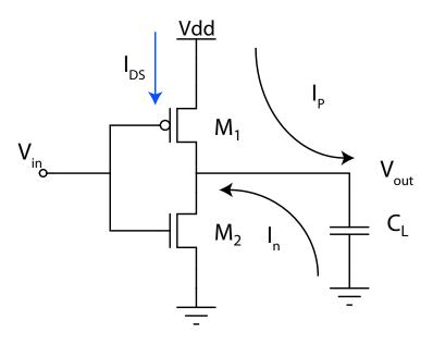
Figure 2.4: Circuit diagram of a CMOS inverter. The switching current is the sum of currents flowing in both the nFET and the pFET.
