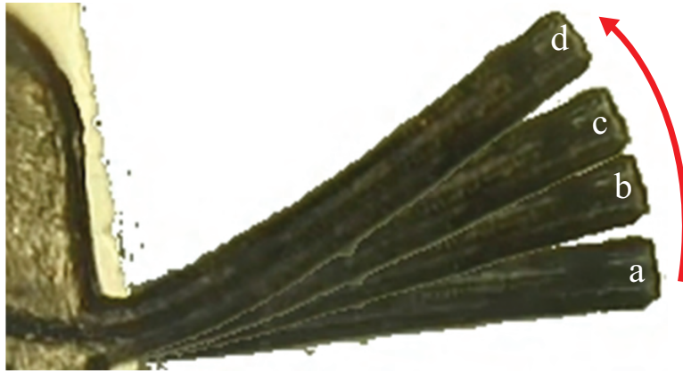
Figure 3.15: Overlaid images of the actuator at a) 0 V, b) 700 V, c) 900 V, and d) 1100 V. The red arrow shows the direction of displacement with increasing voltage.
