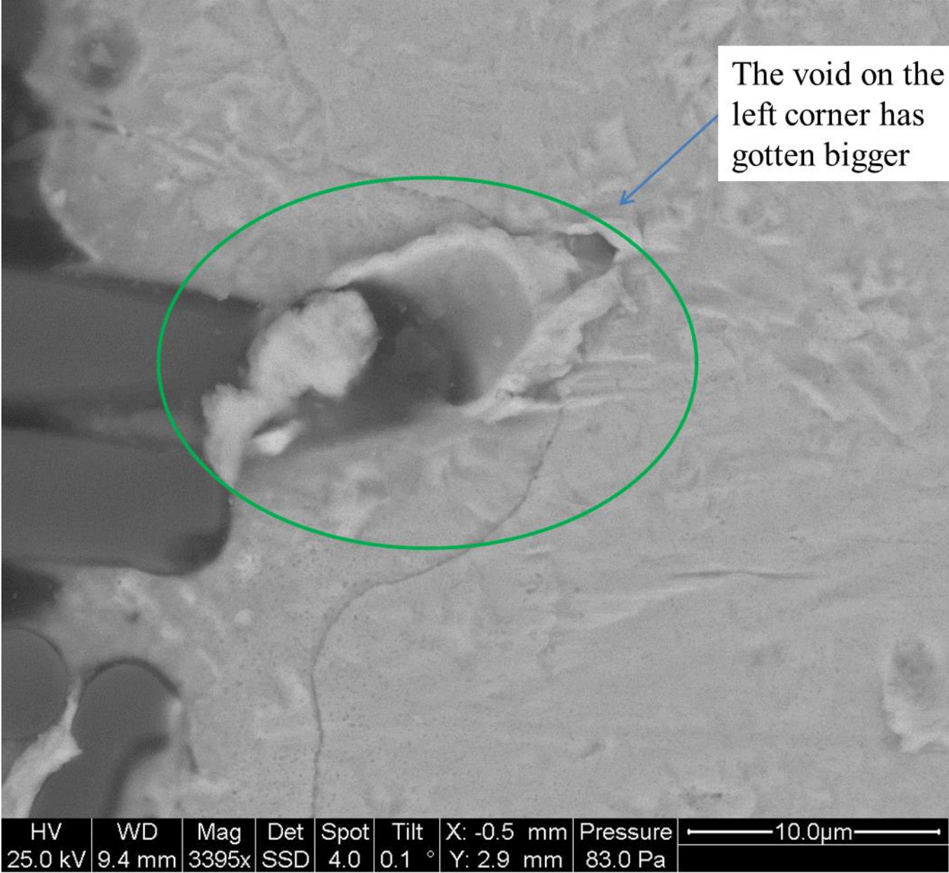
Figure 29- Void expansion after 150 cycle on the single layer microvia
