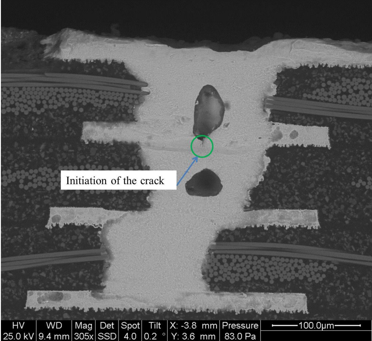
Figure 22-Initiation of the crack at the bottom of the void
